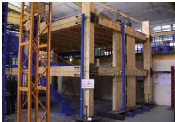
Figure 25: Multi-storey timber building tested at the University of Canterbury (source: Andrew Buchanan)
