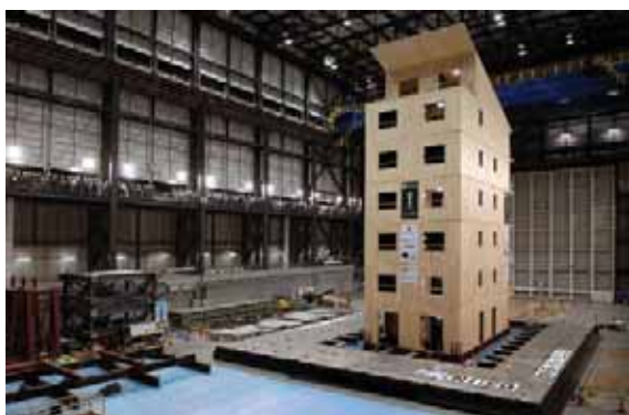
Figure 26: Shake-table testing of a seven-storey CLT building in Japan (source: National Research Council of Italy – Trees and Timber Institute (IVALSA))
