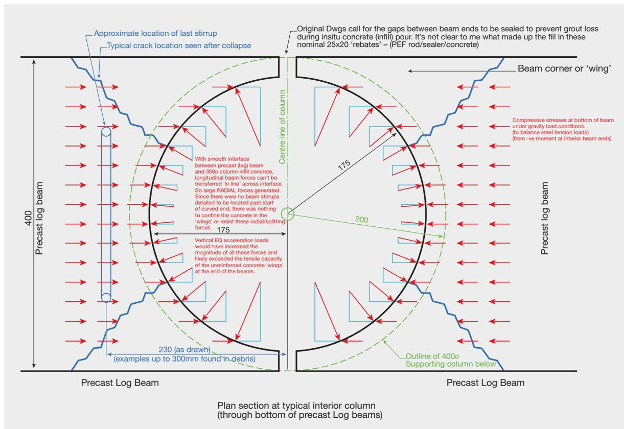
Figure 65: Plan view of beam-column joint prepared by Graham Frost
