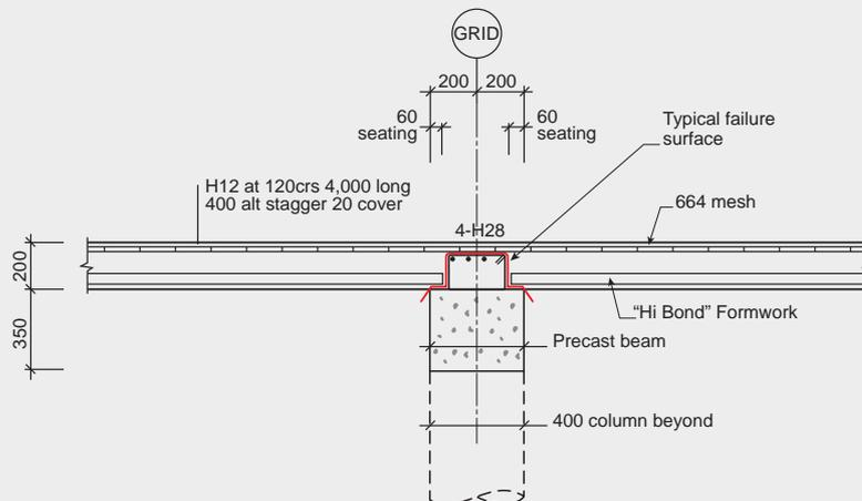
Figure 63(c): Section through precast internal beam to slab with typical observed failure surface indicated in red
