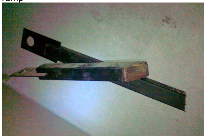
Fractured carstacker top lateral restraints
