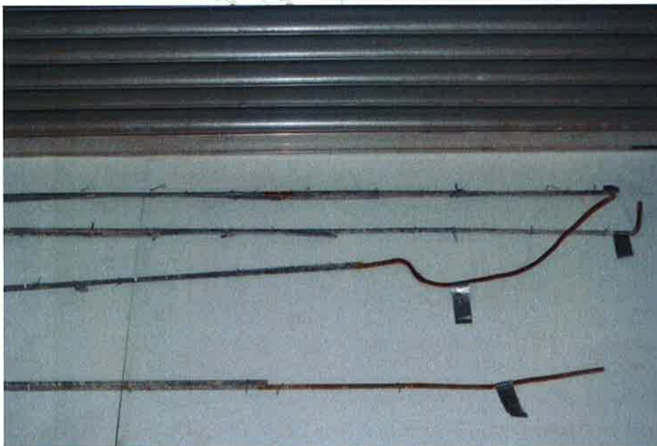
Figure 2 Unprepared 12 mm diameter reinforcing bar samples.
