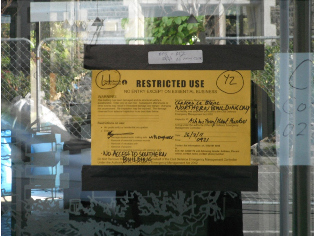
Figure 4-3 A RESTRICTED USE placard with the “Y2” Usability Category indicated in the upper right hand corner. The “L1” in the upper left hand corner probably refers to the fact that the building received a Level 1 Rapid Evaluation at the time of the posting.
