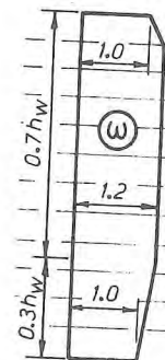
Fig. 6 Dynamic Moment Magnification Factor for Columns in Hybrid Structures.
