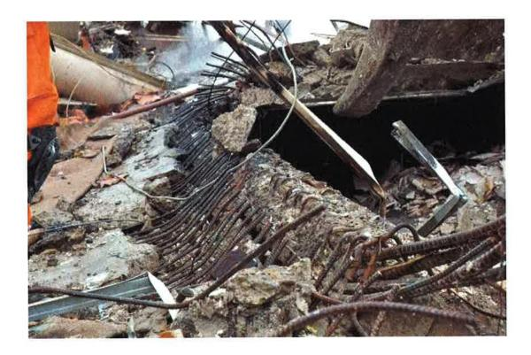
A precast internal beam lying on its side after extraction from the Building. The beam had completely separated from the slab during the collapse as indicated by the fire blackened concrete on the failure surface. The bent bars protruding from the end, the cylindrical surface on the end of the beam and the oxy-cut top reinforcing bars indicate that the end of the beam to the left of the photograph was supported on a round internal column.
