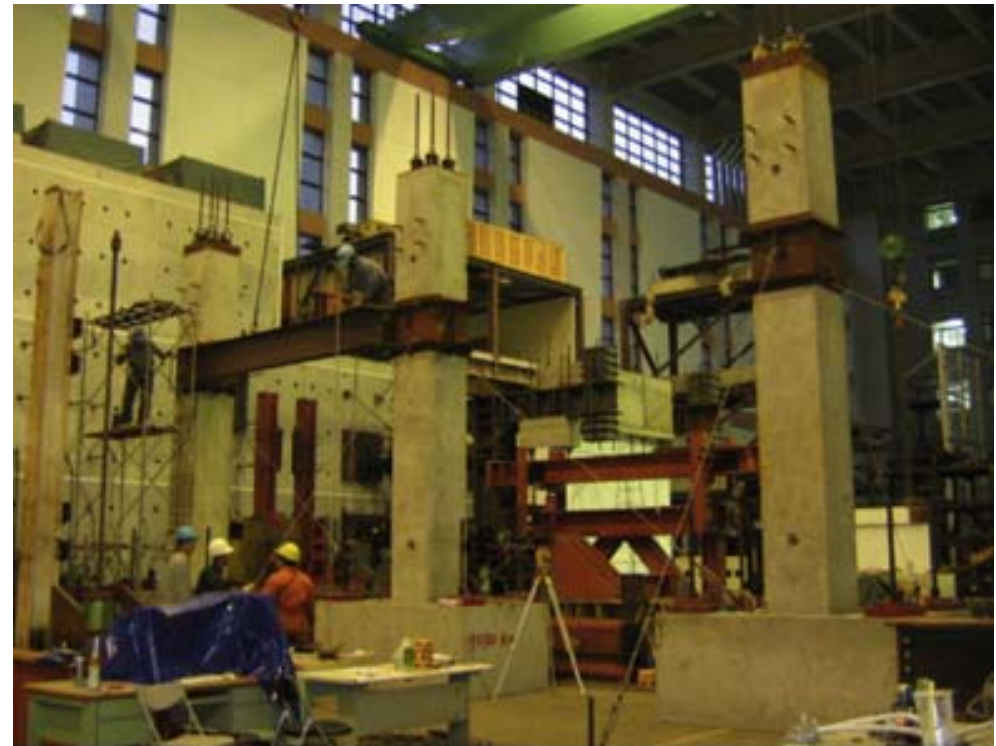
(b) PT beam-column connection and RFP details.
