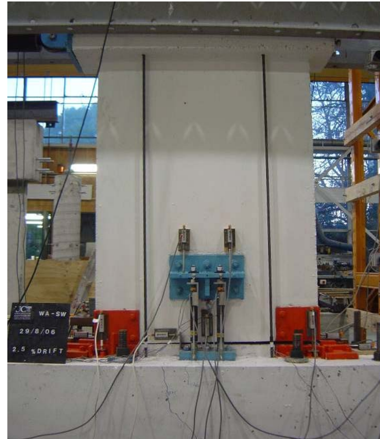
Retrofitted solution using the proposed selective weakening strategy
