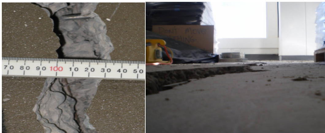
Figure 11: Cold-Drawn Wire Mesh Fracture (left) and Partial Double-T Loss of Seating (right) [31]
