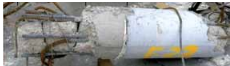
Figure 5.4: Typical 400mm diameter column
