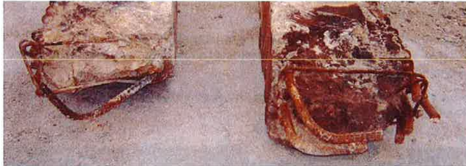
Figure 96 - Interior Pre-cast Log Beams from Line 2 and 3 (DENG Section 3 Dwg S15) showing smooth concrete formed for beam-column joint, and bottom hooked bars that have pulled out of beam-column joints without any obvious straightening;
