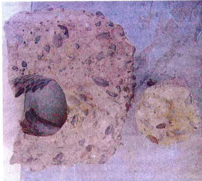
Figure 45 - Concrete from column on Line 4-D/E (C18) showing discolouration from silt.
