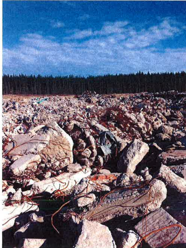
Figure 37 - A portion of the CTV Building debris field at the Burwood Eco Landfill from which columns were extracted for examination and testing.
