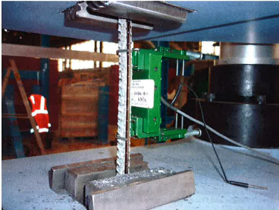
Figure 21 Tensile testing of steel sample
