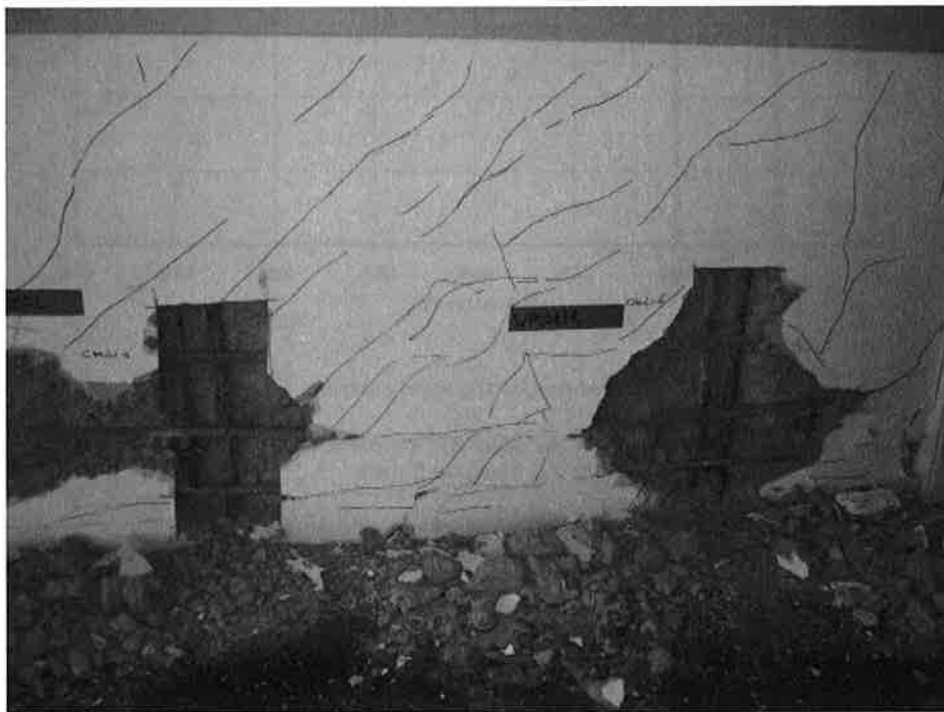
Figure 9 Exposed reinforcing steel in zone of damage in wall element
