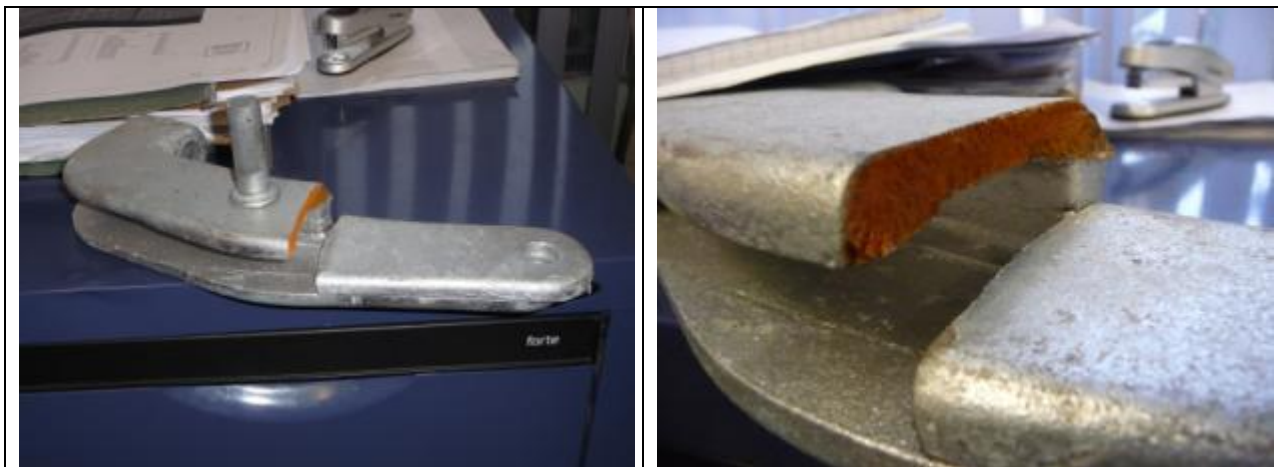
Figure 14: Example of fractured banana end of proprietary brace connector in the roof plane of a long span steel portal frame building [Photos by M. Bruneau]: (a) Global view; (b) Close-up view.
