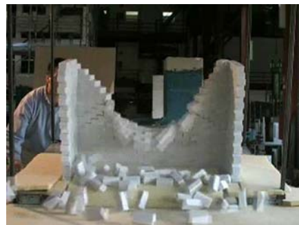
(a) High speed photograph of a dry-stacked masonry wall failing during a tilt test
