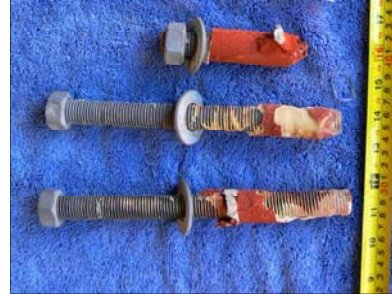
(b) Recovered adhesive anchors that performed inadequately
