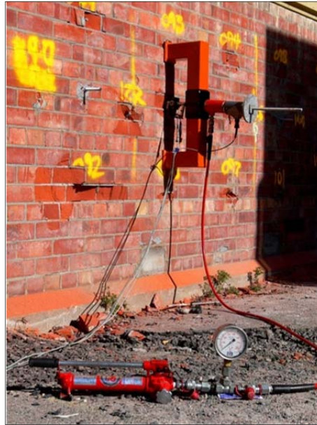
Figure 7.5 Typical test set-up used for pullout anchor testing
