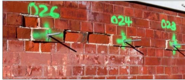
Figure 7.6 Typical masonry pullout type failure observed
