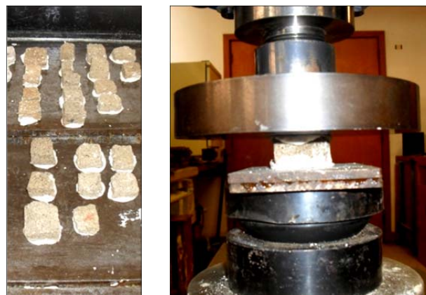
Figure 7.1 Mortar samples and compression test setup
