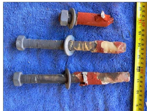
(b) Recovered adhesive anchors that performed inadequately
