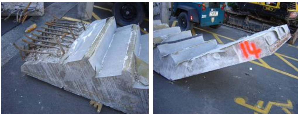
Figure 29 - Unit 14 (Left to right): (a) Mid-height landing bars gas cut; (b) Lower landing intact.
