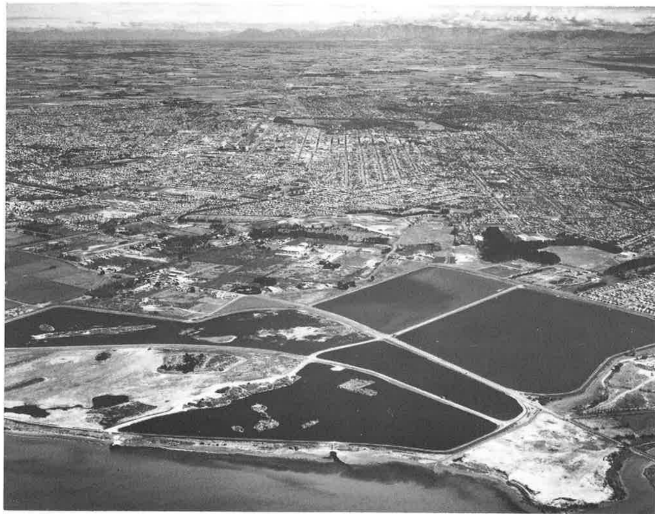
The city of Christchurch occupies a low-lying area of the Canterbury Plains, close to the sea. The plains rise steadily beyond the city to the foothills of the Southern Alps. In the foreground of this 1973 aerial photograph from above the estuary of the Avon and Heathcote Rivers are the oxidation ponds of the city's sewage treatment works. Drainage Board
