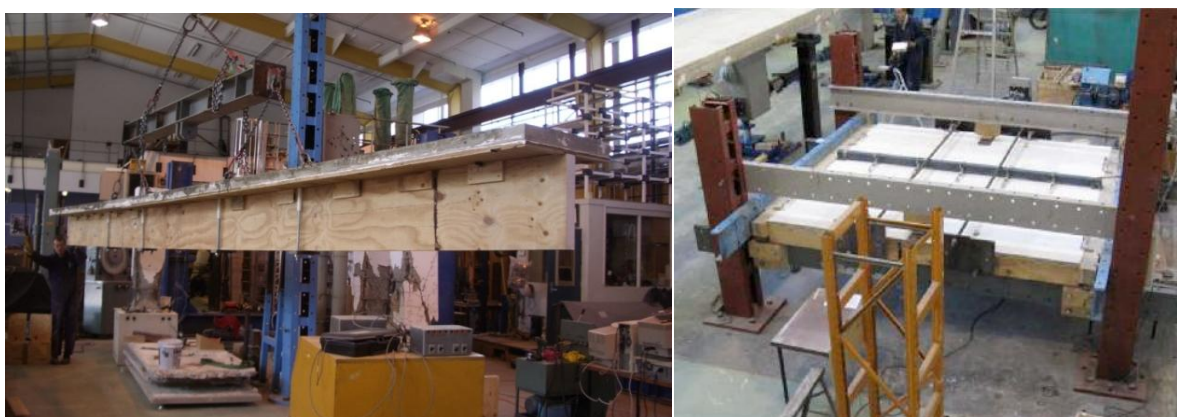
(a) Prefabricated timber-concrete composite floor.
