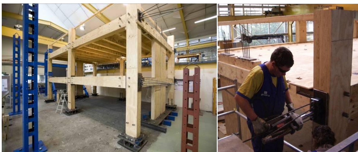
(a) Two-storey post-tensioned frame building after stressing.
