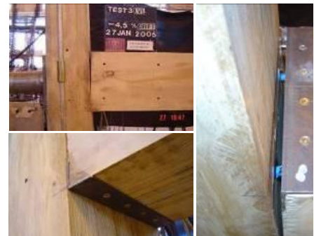
Figure 9.3. Details and performance of post-tensioned timber beam column joints.
