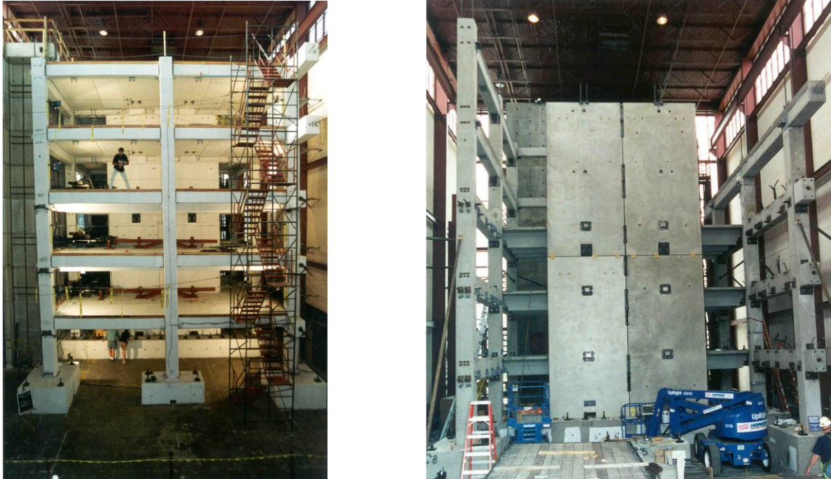
Figure 7.1. Five-Storey PRESSS Building tested at University of California, San Diego (Priestley et al., 1999).
