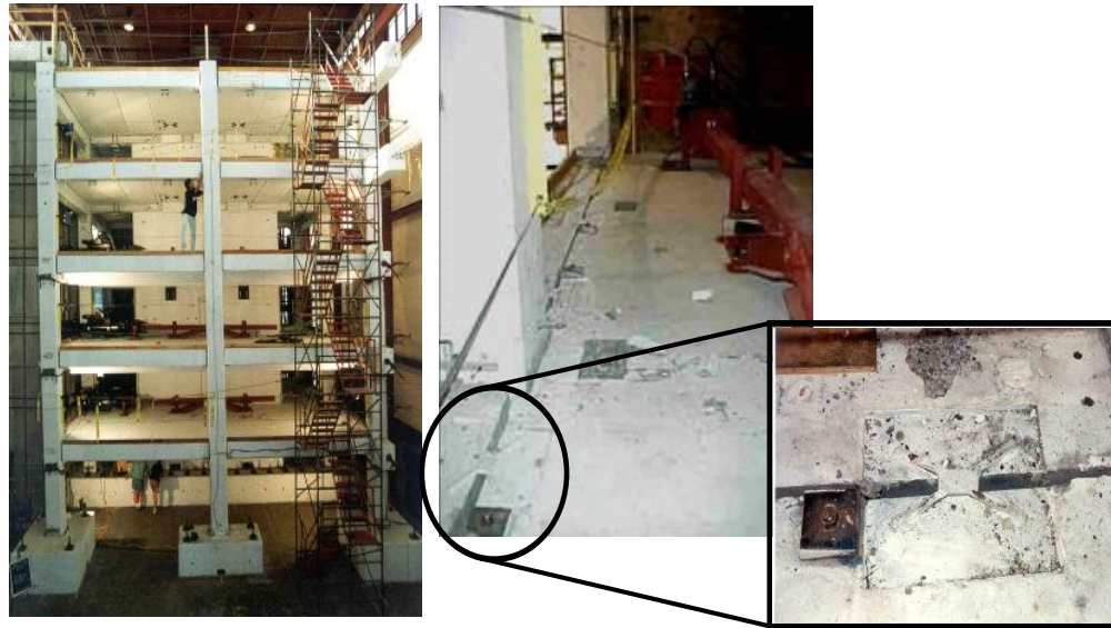
Figure 7.8. Discrete X-plate mechanical connectors used in the PRESSS five storey test building at San Diego (after Priestley et al., 1999).
