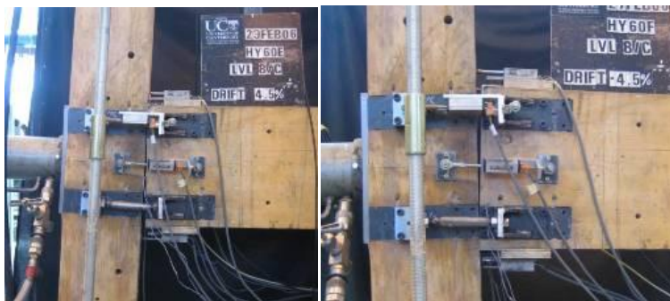
(c) Observed gap opening at 4.5% drift.
