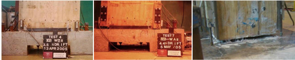
(a) Hybrid walls with three different arrangements of dissipaters.
