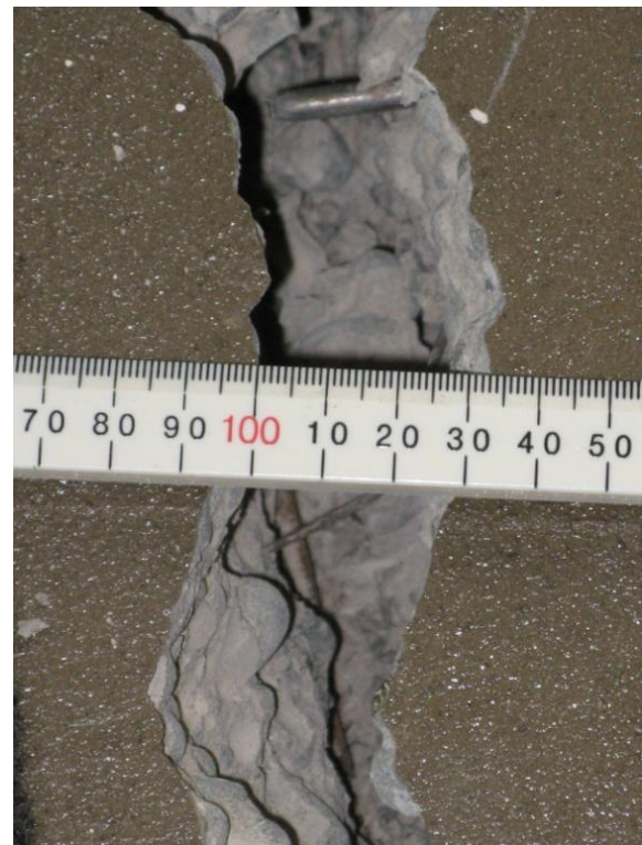
(b) Detail of the crack between the beam and the floor. Cold-drawn wire mesh has fractured.
