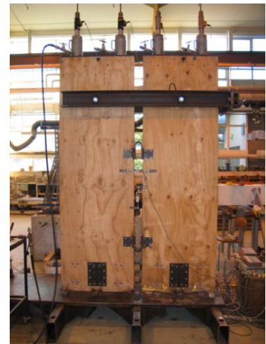
Figure 9.7. Test set-up and coupled wall specimen (Ibqal et al., 2007).
