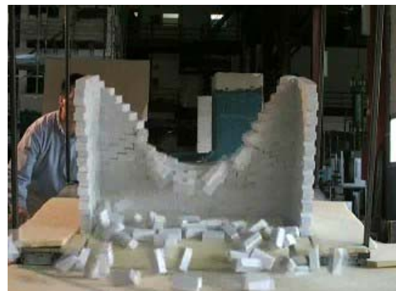
(b) High speed photograph of a dry-stacked masonry wall failing during a tilt test
