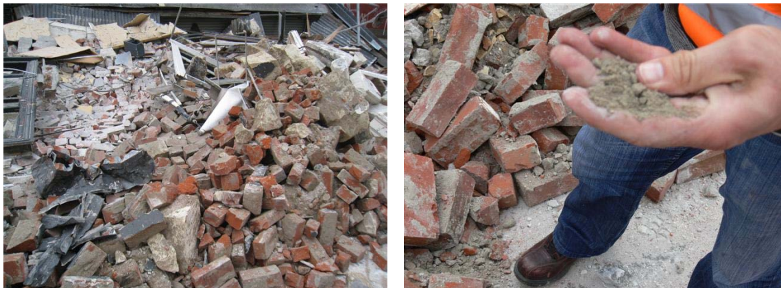
(a) Masonry rubble showing 'clean' bricks
