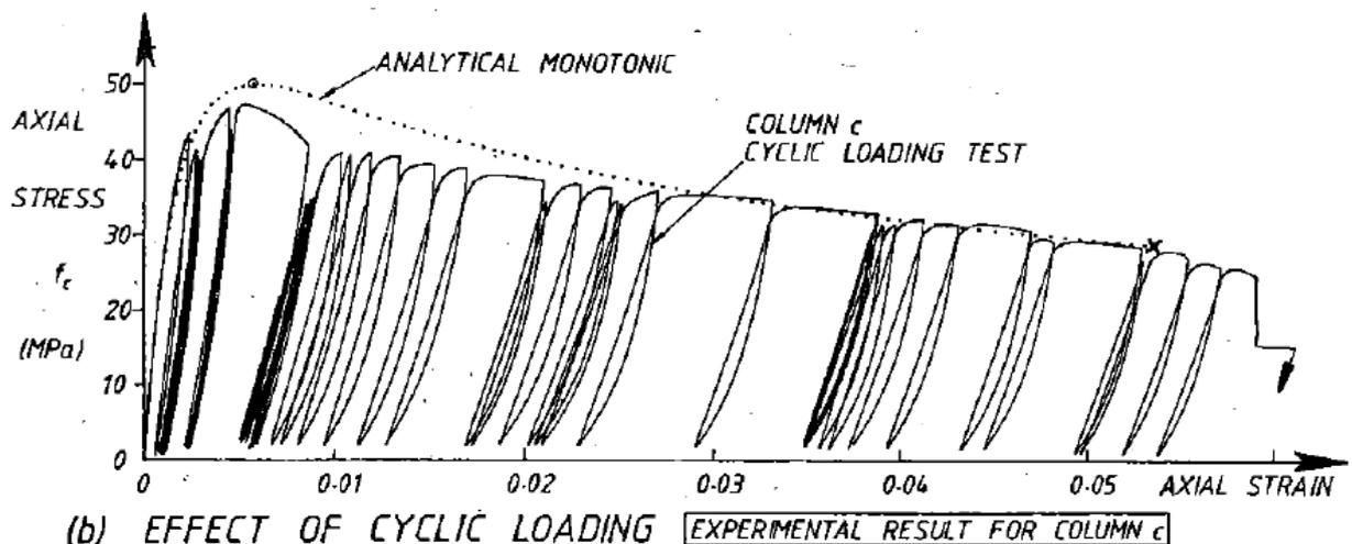
Figure 3. Results of "COLUMN c" tested under compression-only cyclic loading effects by Mander (1983).
