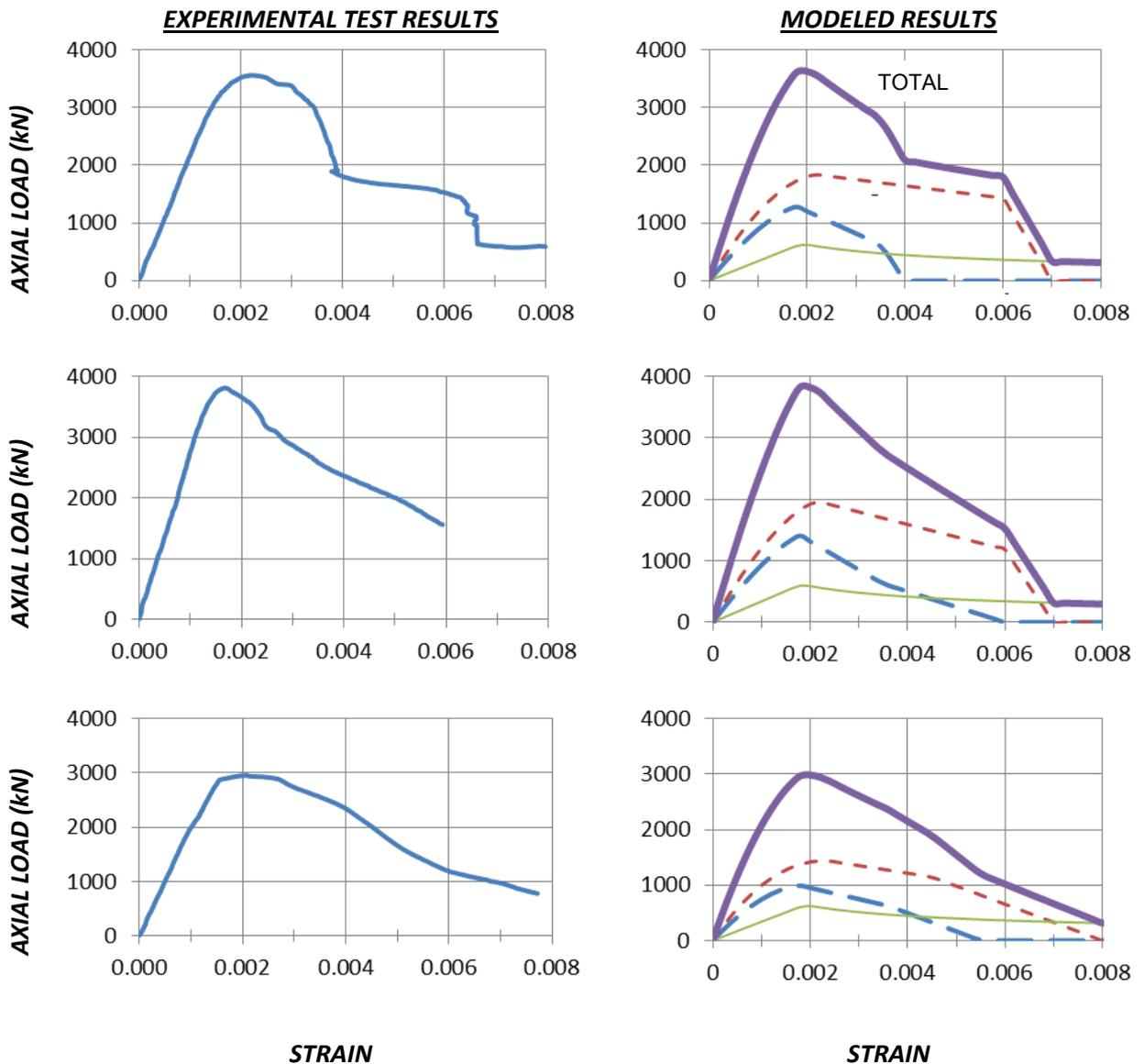
**Figure 1. Experimental test results and the modeling of those results to determine values of the parameters for the stress-strain relations of the in situ concrete.**
