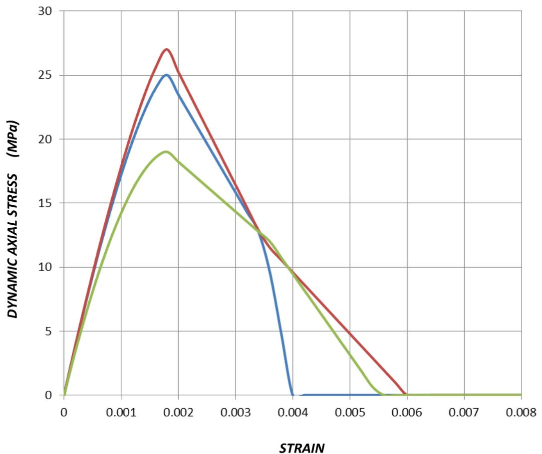
**Figure 2. Inferred stress-strain relations derived from the experimental high-speed test results on the full-scale columns retrieved from the CTV Building.**
