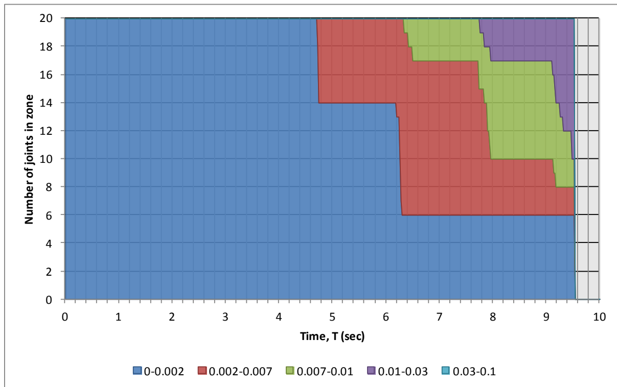
Figure 67: GL A two-way beam-column joint R1 rotations, CBGS, Lyttelton.
