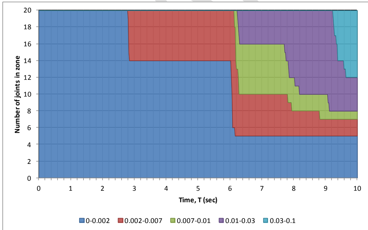
Figure 85: GL A two-way beam-column joint R1 rotations, CHHC, Lyttelton.
