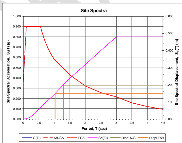
Figure 19: Site spectral displacements.
