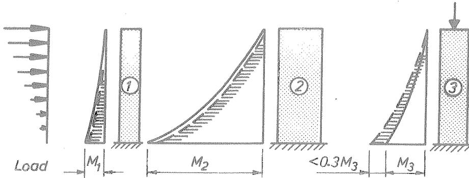
Fig. 11 - Load Redistribution between Three Inelastic Shear Walls.
