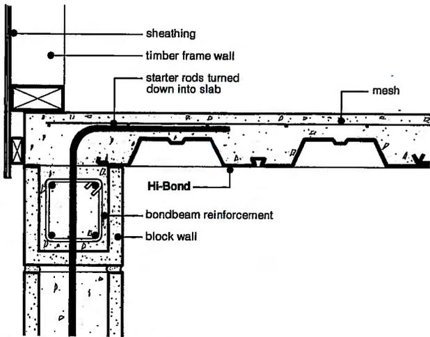
**Fig 3 Masonry wall support with timber wall above**
