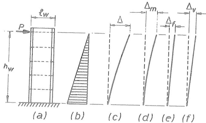
Fig. 28 - A Cantilever Wall and its Distortions.
