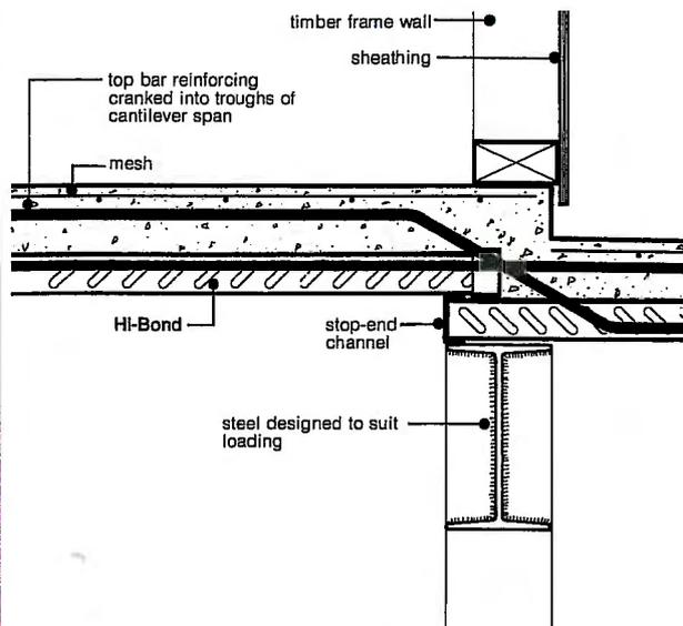
**Fig 11 Cantilever — steel beam support**
