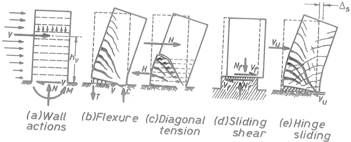
Fig. 1 - Possible Failure Modes in Cantilever Shear Walls
