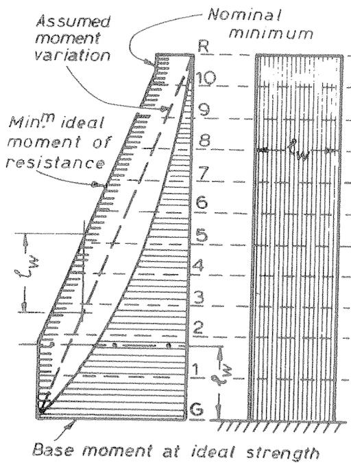
Fig. 15 - Recommended Design Bending Moment Envelope for Cantilever Shear Walls.
