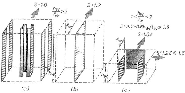
Fig. 2 - Types of Cantilever Shear Walls with Appropriate S Factors
