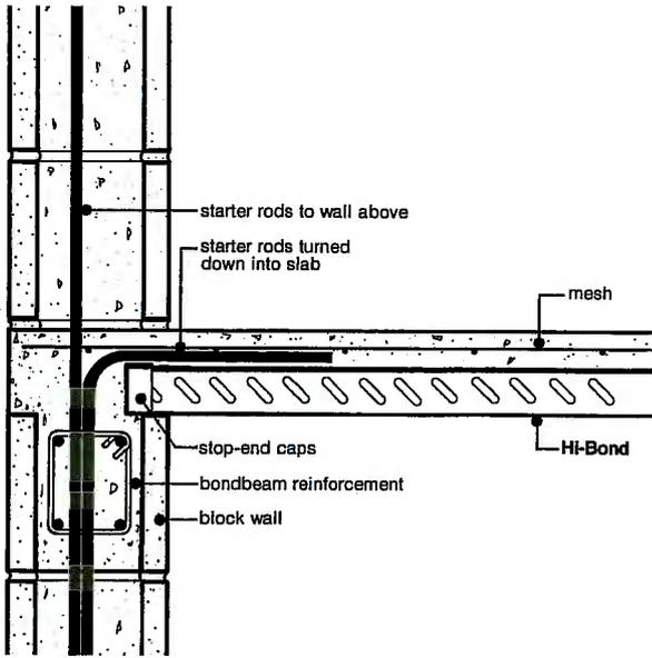
**Fig 1 Masonry wall support with masonry wall above**
