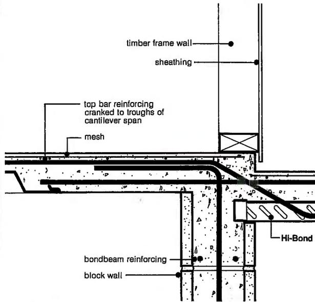
**Fig 7 Cantilever — masonry wall**
