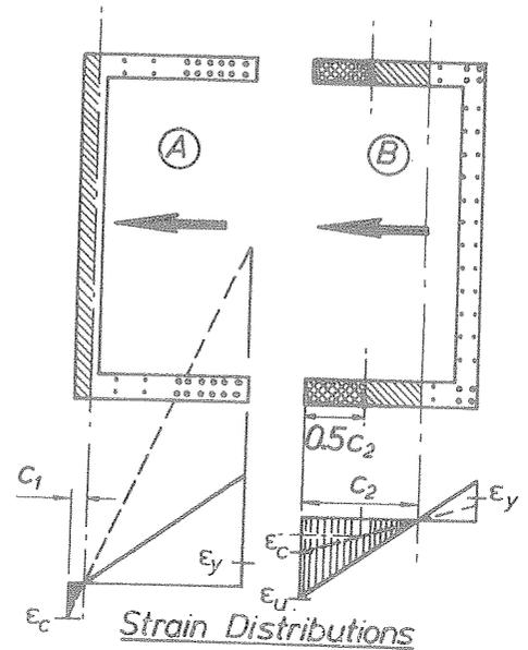
Fig. 22 - Strain Profiles for Channel Shaped Wall Sections.
