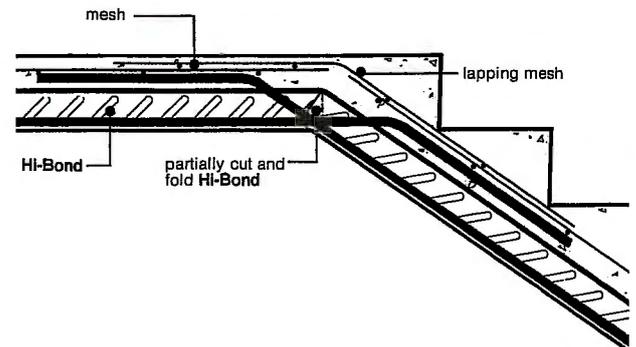
**Fig 12 Typical stair detail**
