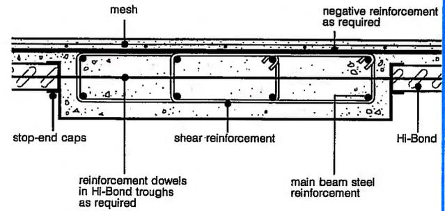
**Fig 4 Concrete beam support**
