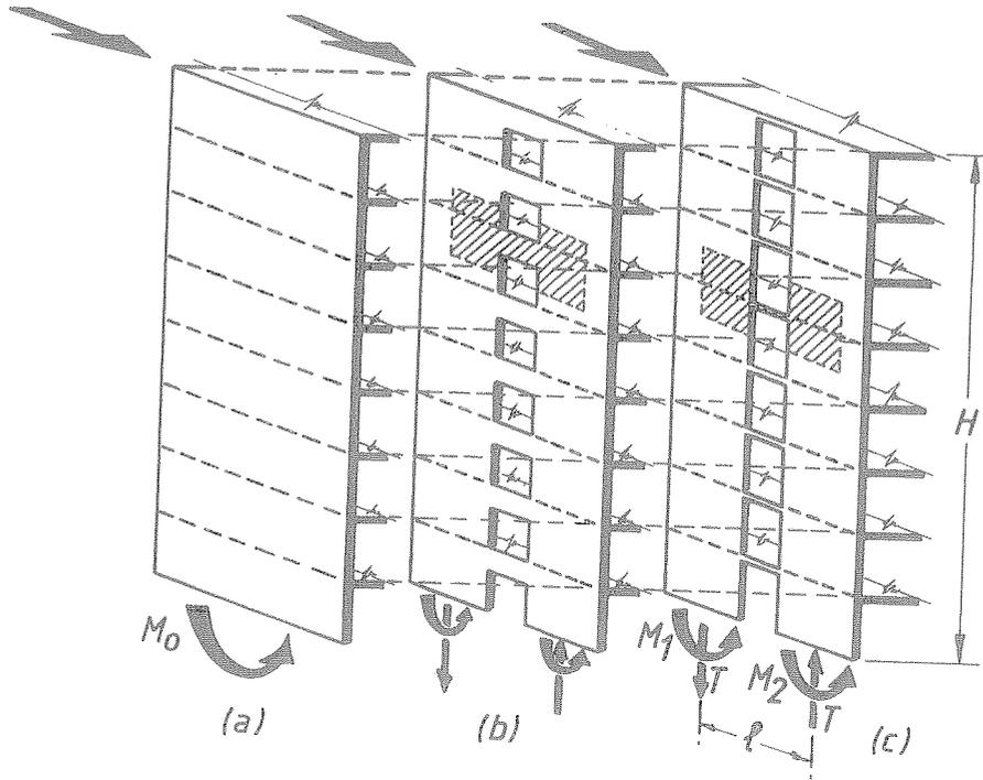
Fig. 17 - A Comparison of Ductile Walls (a) A Cantilever Wall (b) Wall Coupled by Strong Coupled Beams (c) Walls Coupled by Slabs Only
