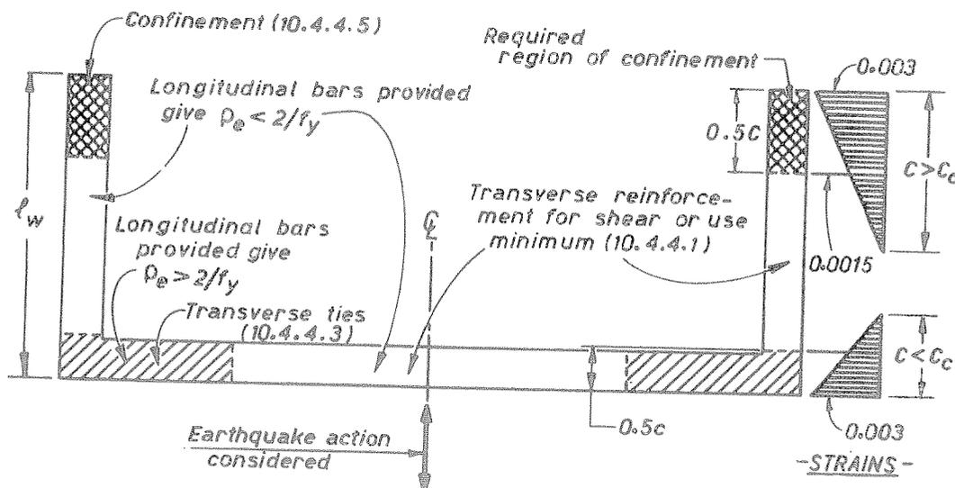
Fig. 24 - Regions of Different Transverse Reinforcement in a Shear Wall Section.
