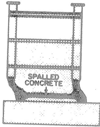
Fig. 25 - Sliding Shear Failure Initiated by Web Crushing.
