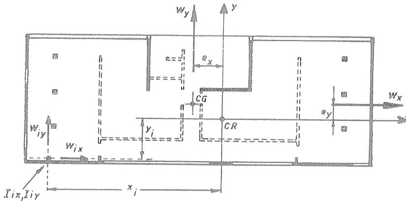
Fig. 12 - Shear Wall Layout for an Apartment Building (2)
