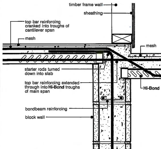
**Fig 9 Cantilever — masonry wall**
