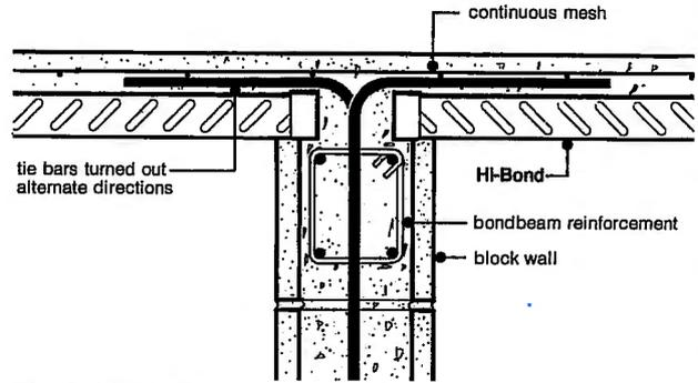
**Fig 2 Typical internal wall**
