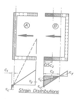
Fig. 22 - Strain Profiles for Channel Shaped Wall Sections.
