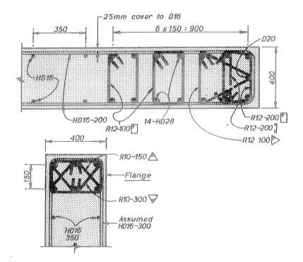
Fig. 36 - Arrangement of Transverse Reinforcment in the Critical Regions of the Example Shear Wall Section.
