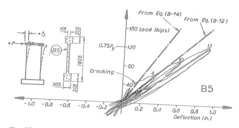
Fig. 33 - Continuous Load-Deflection Plot for the Initial Cycles for Specimen B5.
