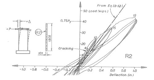
Fig. 32 - Continuous Load-Deflection Plot for Initial Cycles for the Rectangular Wall Specimen R2.
