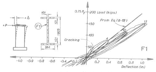
Fig. 31 - Continuous Load-Deflection Plot for Initial Cycles for the Flanged Wall Specimen Fl.
