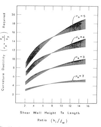
Fig. 16 - The Variation of Curvature Ductility at the base of Cantilever Shear Walls with the Aspect Ratio of the Walls and the Imposed Displacement Ductility Demand (14).
