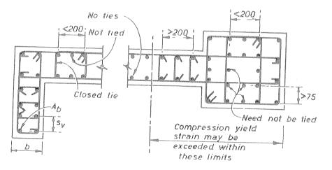
Fig. 23 - Transverse Reinforcement in Potential Yield Zones of Shear Wall Sections.
