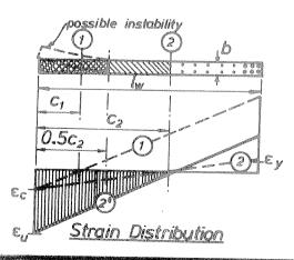
Fig. 20 - Strain Patterns for a Rectangula Wall Section Subjected to Flexure and Axial Load.
