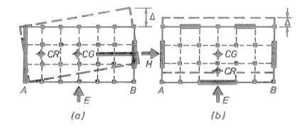
Fig. 13 - The layout of Shear Walls affects the Torsional Stability of the Lateral Load Resisting System.
