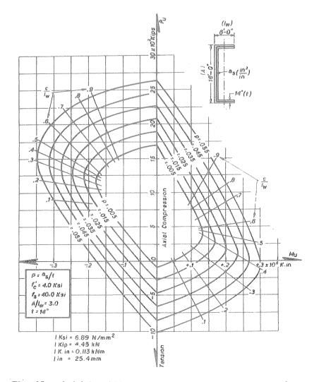
Fig. 10 - Axial Load-Moment Interaction Curves for a Channel Shaped Wall Section (2)
