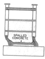
Fig. 25 - Slidng Shear Failure Initiated by Web Crushing.
