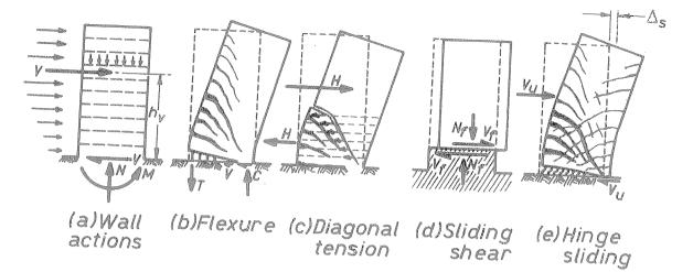
Fig. 1 - Possible Failure Modes in Cantilever Shear Walls
