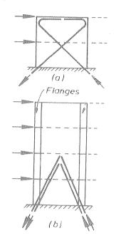
Fig. 26 - Suggestions for the Arrangement of Diagonal Reinforcement to Control Slidng Displacement at the Base.
