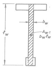
Fig. 29 - Effective Shear Area of a Flanged Wall Section.
