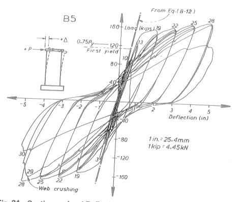
Fig. 34 - Continuous Load-Deflection Plot for all Cycles for Specimen B5
