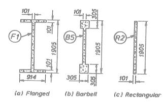
Fig. 30 - Nominal Cross Sectional Dimensions of the PCA Test Specimens (11).
