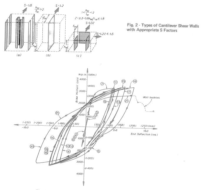
Fig. 3 - Load-Displacement Response to Cyclic Reversed Loading of a Ductile Shear Wall Structure (10)
