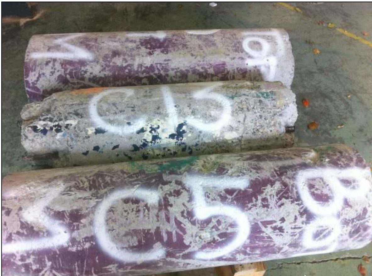
Figure 2.4. The three column portions retrieved from the CTV Building used in the full-scale testing conducted at the University of Canterbury
