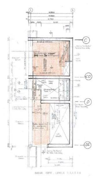
Diagram 5 showing Shear Core North Wall. Shaded areas show connection of slab to rear of wall line (5). The areas with cross lines are opening for stairs, lifts and ducts
