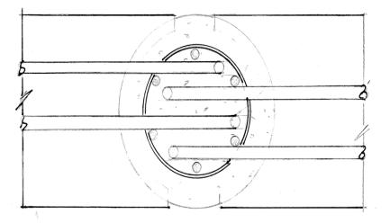
Diagram 3: shows a horizontal section through the beam column joint
