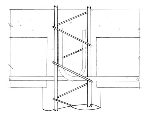
Diagram 2 shows a vertical section through the beam column joint. Note: effectively one tie 6 mm in diameter that is placed in the joint. The bent up bars from the precast beams have limited anchorage in the joint zone.
