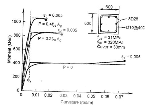
Figure 7.13: Moment curvature response of unconfined columns
