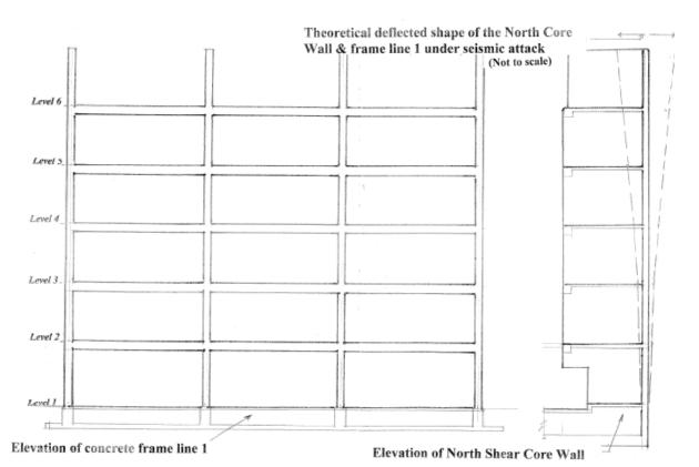
Diagram 4 showing frame line F with North Shear Core. The frame is joined to the shear wall by the slab. Note the notice in the base of the wall. The columns in frame line F have not been detailed for ductile action.
