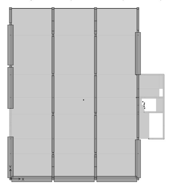
Diagram 1: Plan of building showing the centre of mass as the dot in the centre of the floor plate and the centre of stiffness shown as the collection of dots in the North Core wall (stair well)
