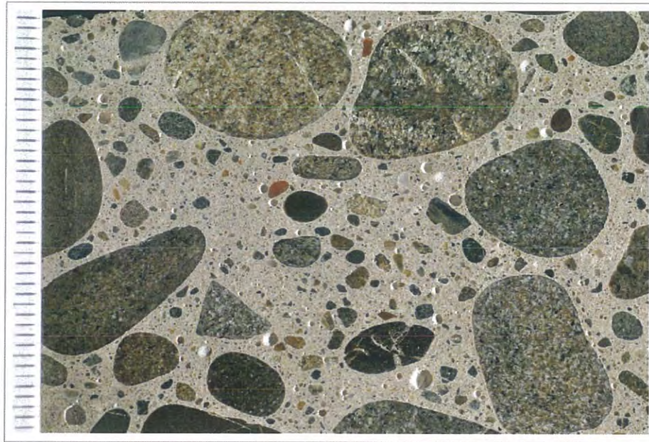
Figure E4. Photograph of the polished surface showing coarse aggregate; scale in millimeters.
