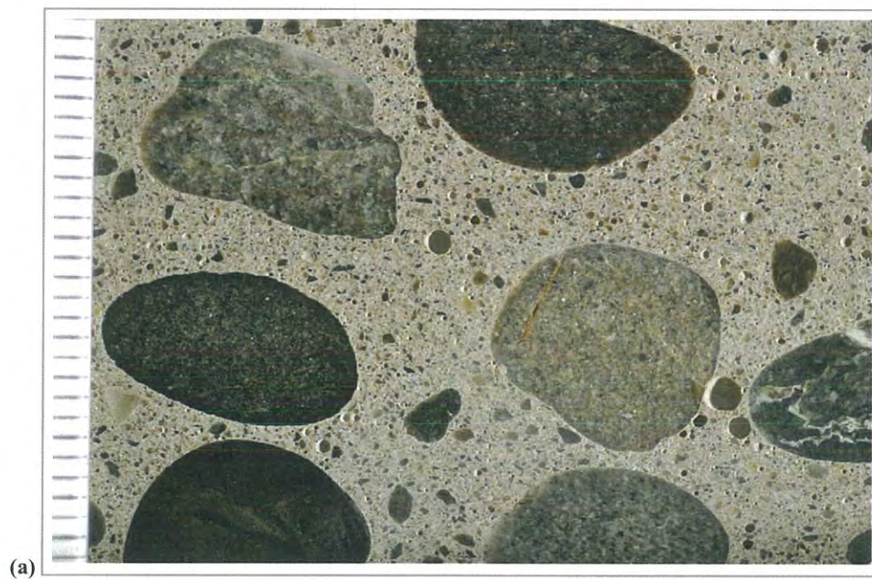
Figure H6. (a) Photograph of the polished surface from the top portion of the core showing coarse aggregate; scale in millimeters.
