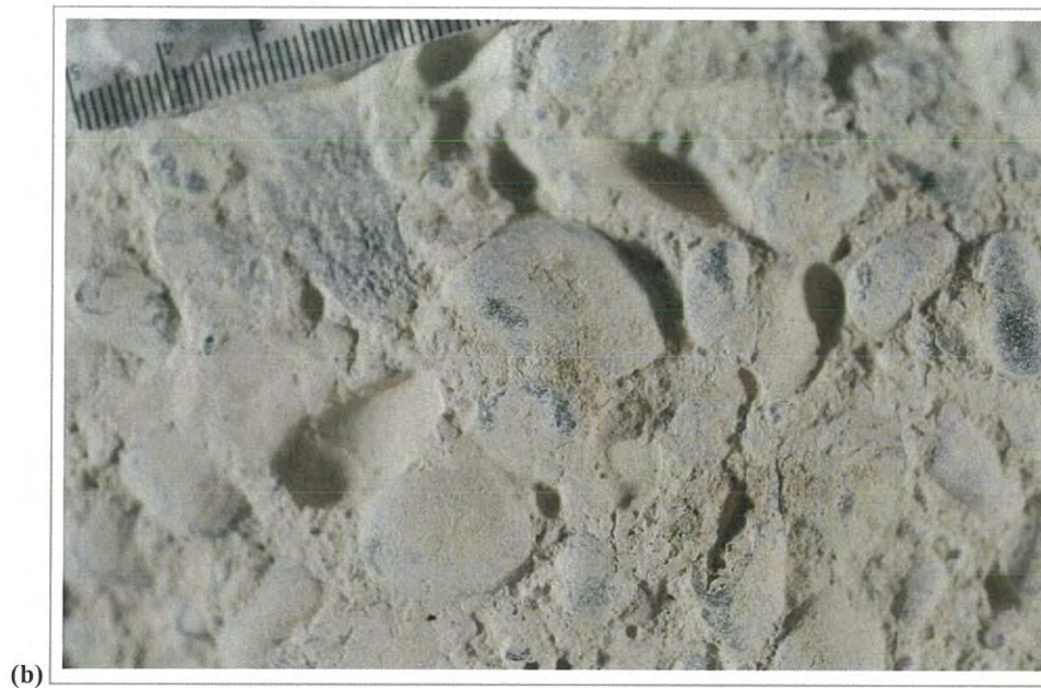
Figure A3 (cont'd). Photograph showing detail of the bottom surface of the core; scale in millimeters.
