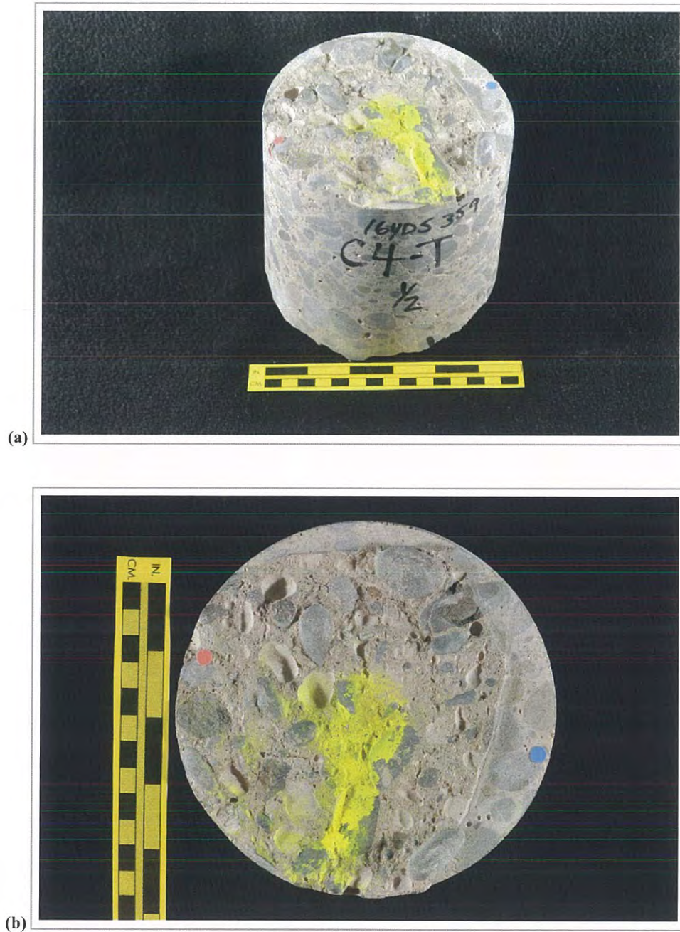
Figure D1. Photographs showing (a) oblique view of the top and side of the core with identification labels and (b) the top of the core. The red and blue dots show the orientation of the saw cuts used to prepare the sample.
