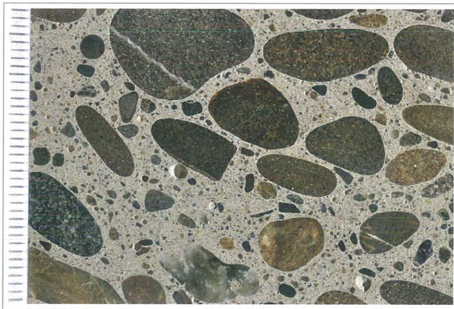
Figure B6. Photograph of the polished surface showing coarse aggregate; scale in millimeters.
