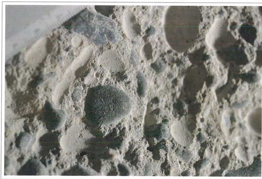
Figure C3. Photograph showing detail of the bottom as-received fracture surface; scale in millimeters.
