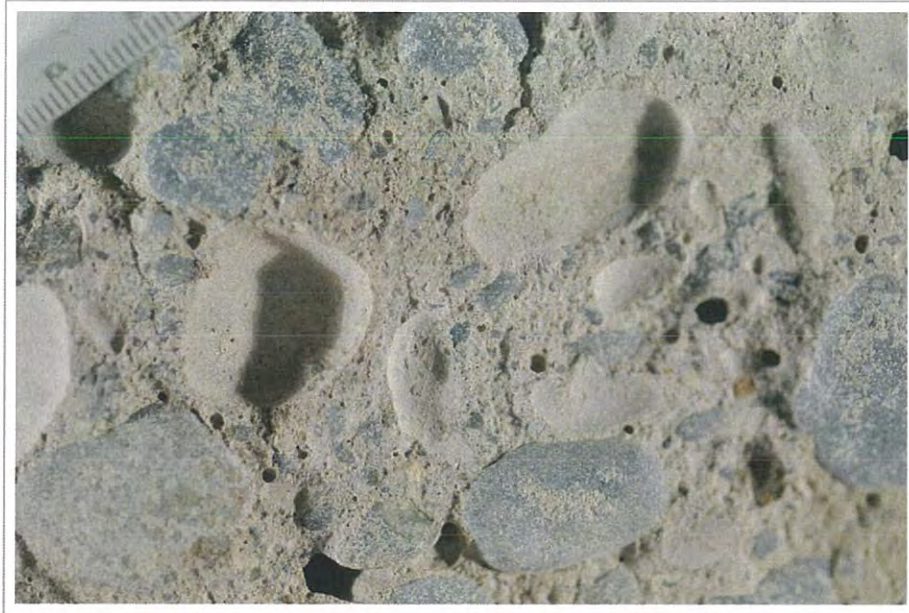
Figure D3. Photograph showing detail of the top fracture surface of the core; scale in millimeters.
