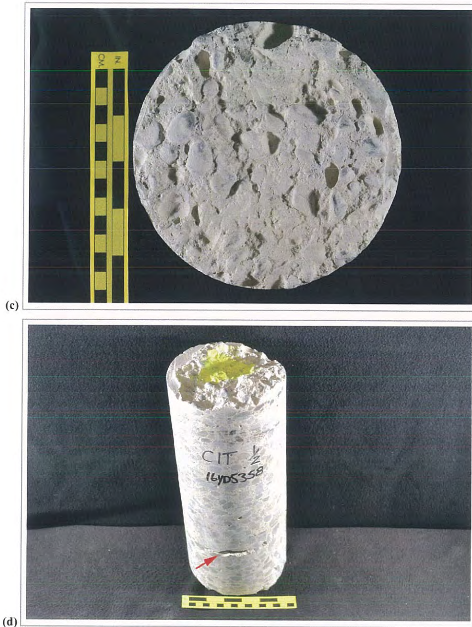
Figure B1 (cont'd). (c) Photograph showing the bottom surface of the core. (d) Photograph showing both sections of the core designated as C1-T ½. The section that was the subject of the petrographic examination represented the lower portion of the core. The red arrow highlights the crack that separated the top and lower portions of the core.
