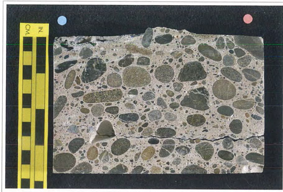
Figure C2. Photograph showing one of the polished surfaces of the core.
