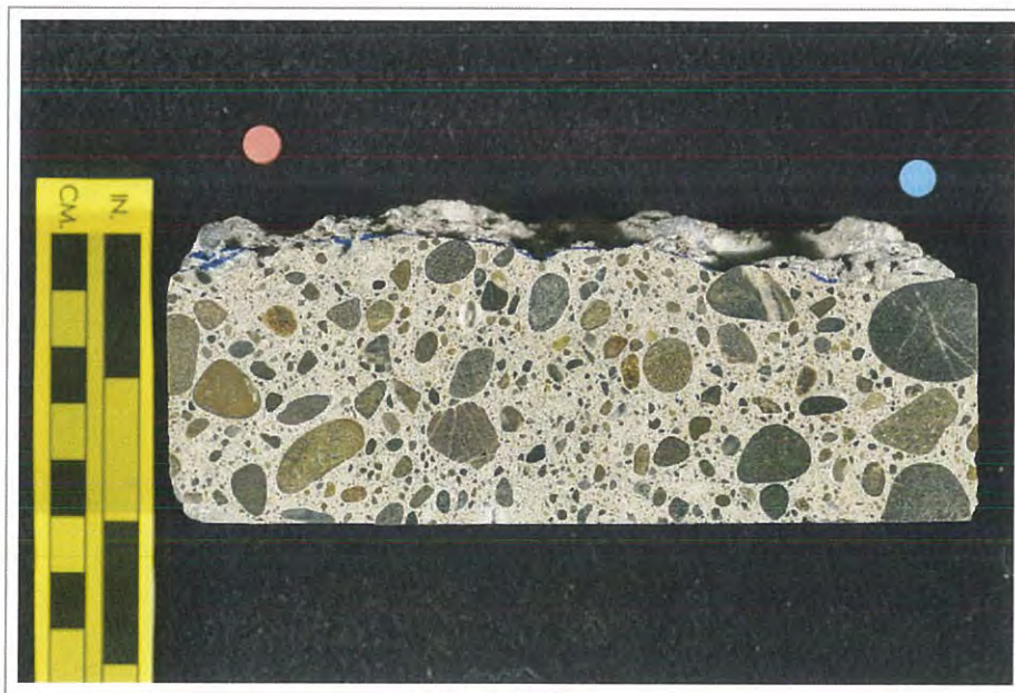
Figure F3. Photograph of one of the polished surfaces used for petrographic work.
