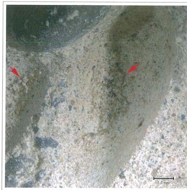
Figure A9. Reflected light photomicrograph of a fresh fracture surface showing two aggregate sockets that contained sand grains (red arrows).
