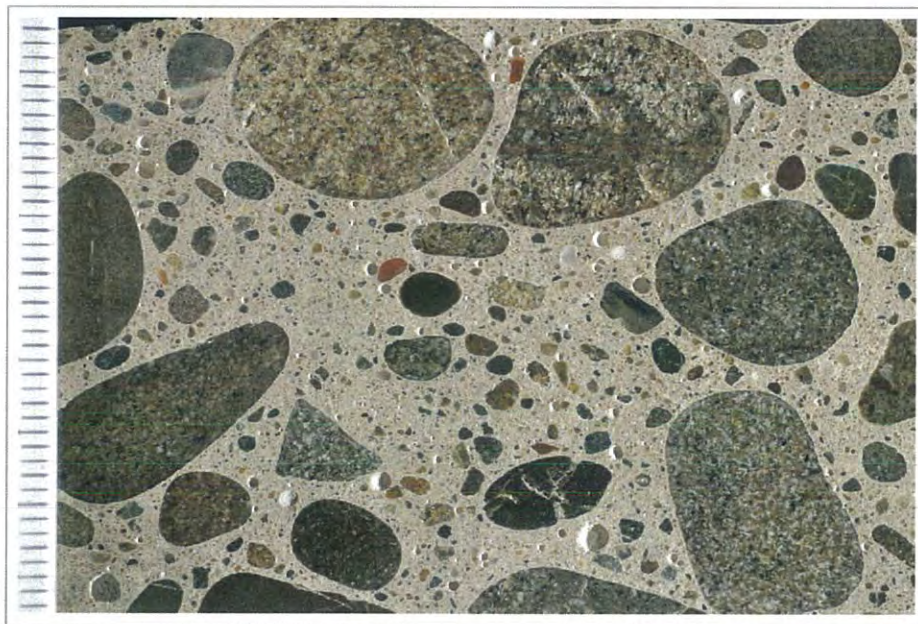
Figure C6. Photograph of the polished surface showing coarse aggregate; scale in millimeters.
