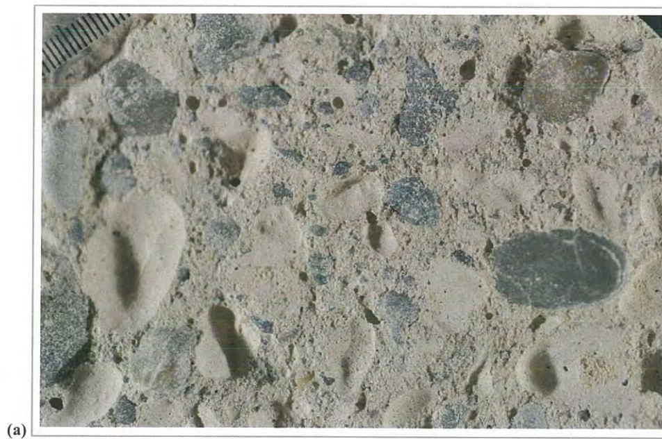
Figure B3. Photograph showing detail of the top surface of the core; scale in millimeters.
