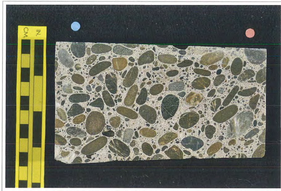
Figure E2. Photograph showing one of the polished surfaces of the core.
