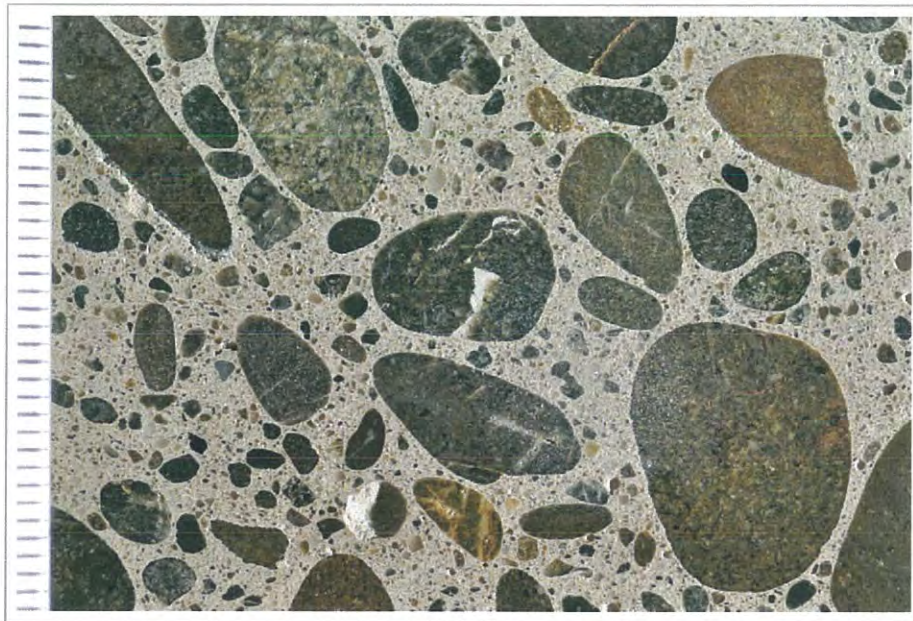
Figure A5. Photograph of the polished surface showing coarse aggregate; scale in millimeters.
