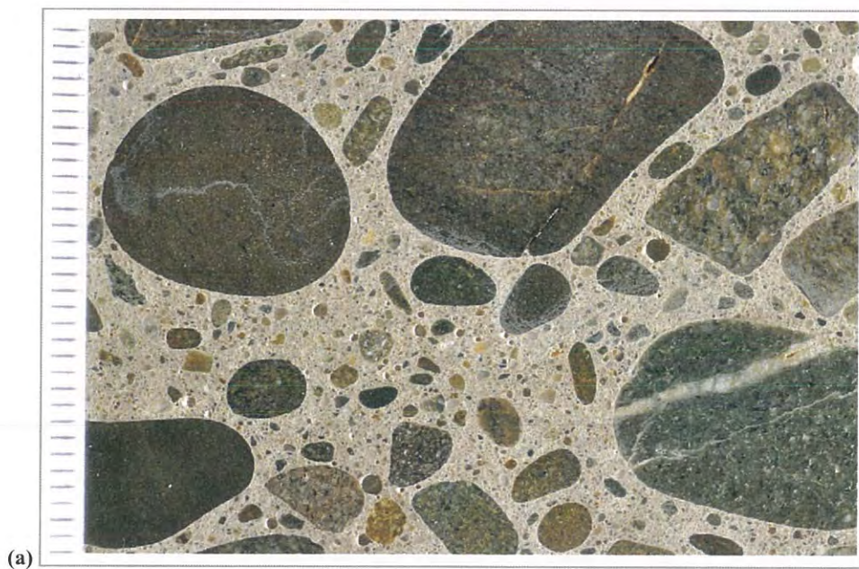
Figure D6 (cont'd). Photograph of the polished surface showing coarse aggregate; scale in millimeters.
