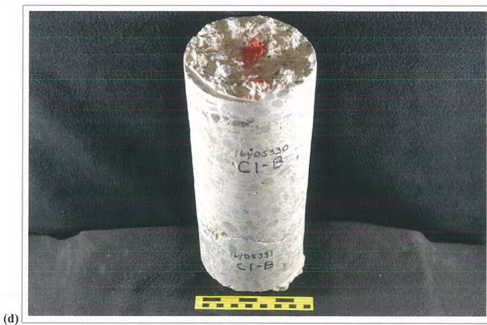
Figure A1 (cont'd). (c) Photograph showing the bottom surface of the core. (d) Photograph showing both sections of the core designated as C1-B. The section that was the subject of the petrographic examination represented the lower portion of the core.
