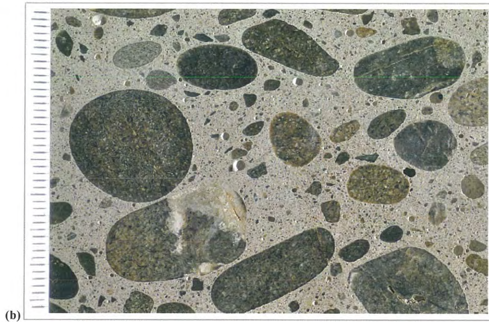
Figure H6 (cont'd). (b) Photograph of the polished surface from the bottom portion of the core showing coarse aggregate; scale in millimeters.
