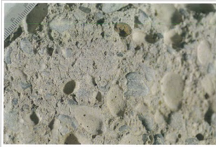
Figure F2. Photograph showing detail of the top surface of the core; scale in millimeters.
