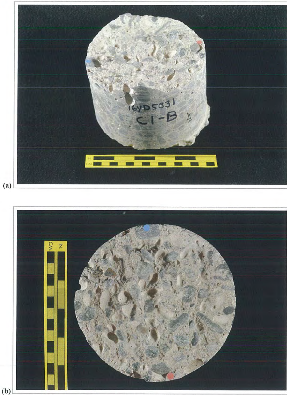
Figure A1. Photographs showing (a) oblique view of the top and side of the core with identification labels and (b) the top of the core. The red and blue dots in (a) show the orientation of the saw cuts used to prepare the sample.
