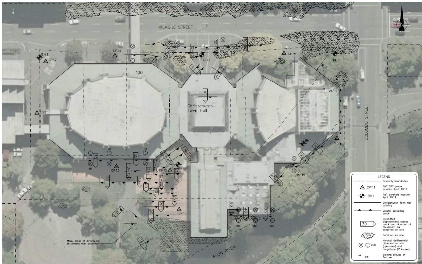
Figure 17: Lateral Spreading Map [5]
