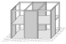
(a) Shear walls
