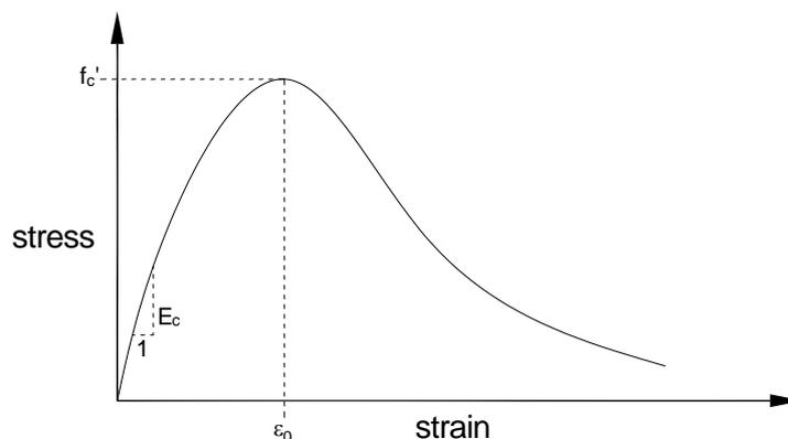
**Figure 5: Concrete stress-strain curve**
