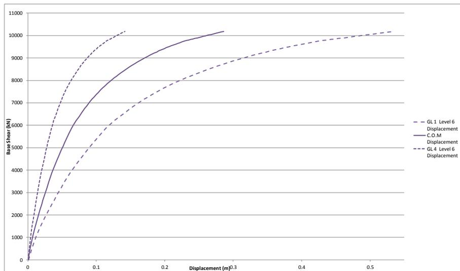
**Figure 32: Model A Level 6 eastern pushover displacement profile.**
