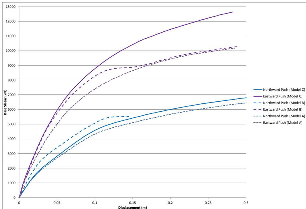
**Figure 36: Pushover force displacement variations for north and east directions.**
