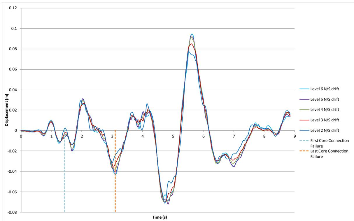
**Figure G.3: Frame A north/south inter-storey displacements.**
