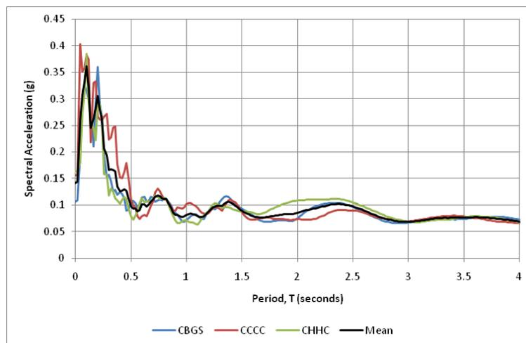
**Figure 23: Darfield Vertical 5% damped response spectra**
