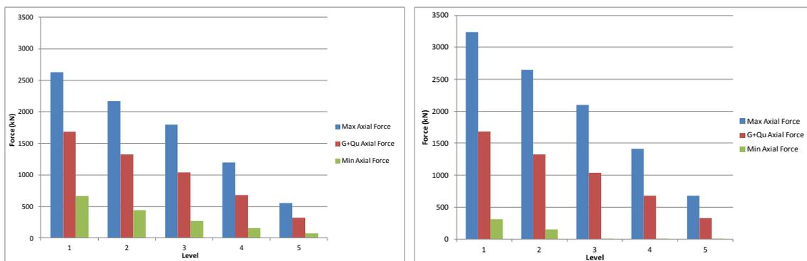
**Figure 52: Column D2 axial load variation - CBGS (left) & CCCC (right), Lyttelton**
