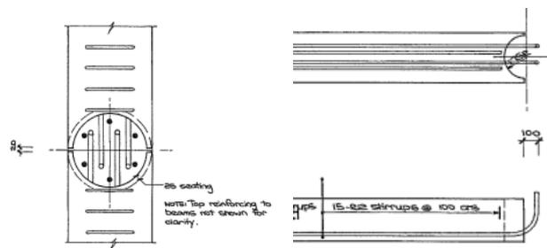
**Figure 12: Typical bottom reinforcement anchorage in interior beam column joint zone [1]**
