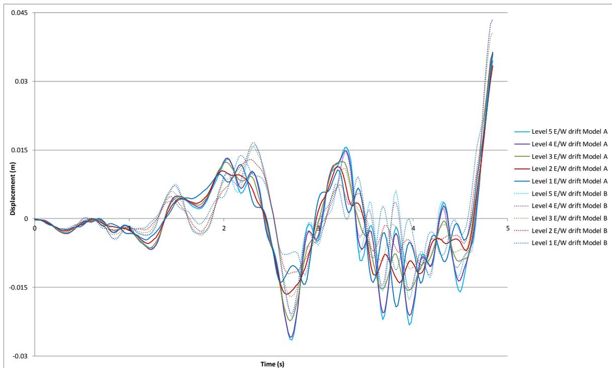
**Figure I.5: Frame 1 east/west inter-storey displacements.**
