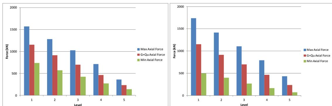
**Figure 53: Column F2 axial load variation - CBGS (left) & CCCC (right), Lyttelton**
