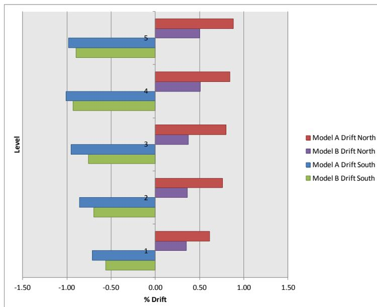
**Figure 38: Frame A north/south storey drifts - Darfield.**
