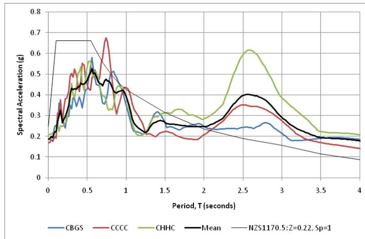
**Figure 21: Darfield N00E 5% damped response spectra (north/south)**
