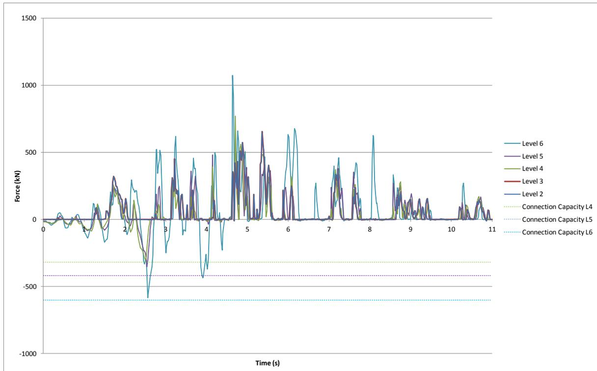
**Figure F.12: North core Wall D diaphragm north/south actions.**
