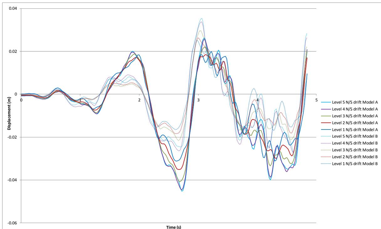
**Figure I.3: Frame A north/south inter-storey displacements.**
