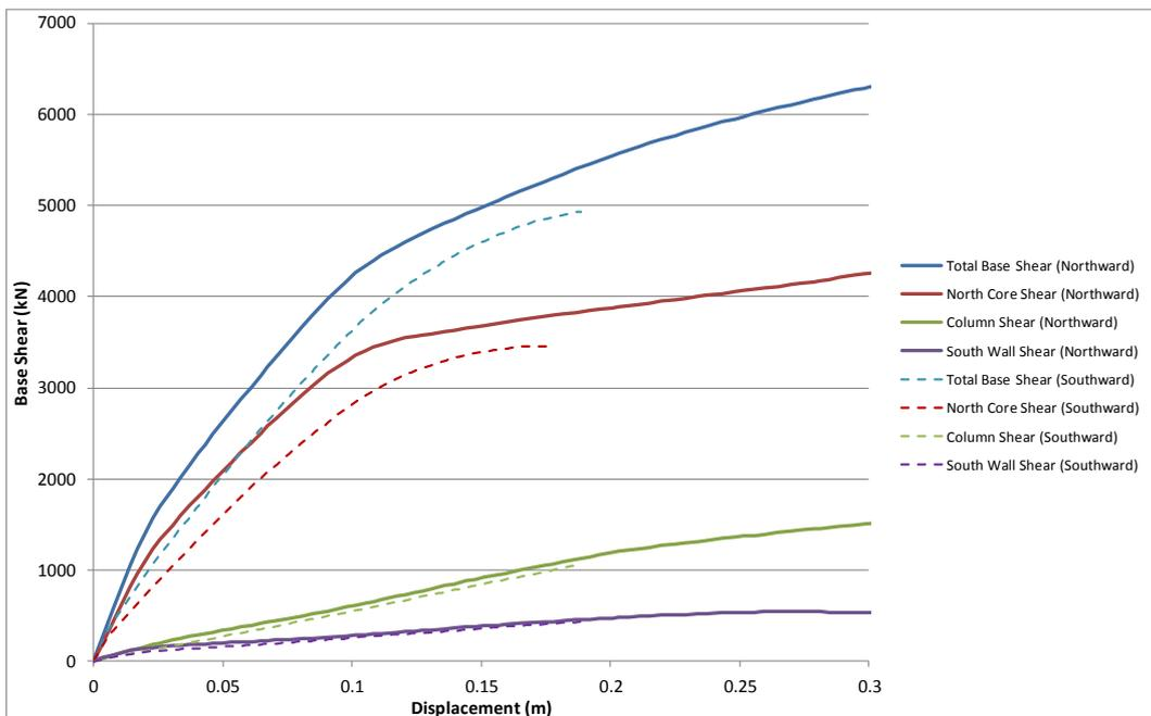
**Figure 30: Model A base shear components - north/south direction.**
