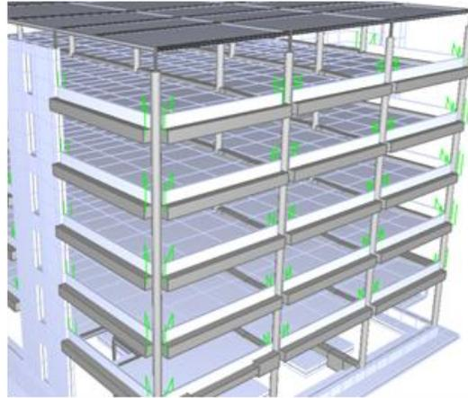
**Figure 18: Model C screenshot showing spandrel panels.**
