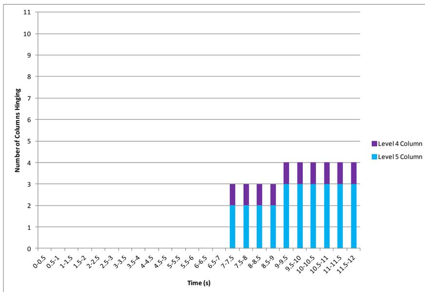
**Figure 44: Column hinge progression - Darfield, Model B.**
