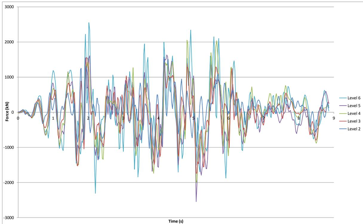
**Figure G.15: North core Slab 4/C to C/D diaphragm east/west actions.**
