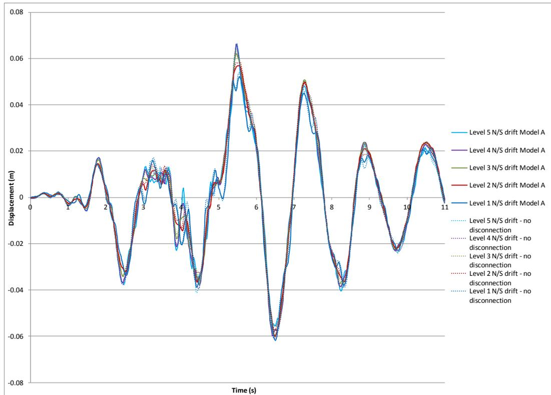
**Figure J.4: Frame F north/south inter-storey displacements.**
