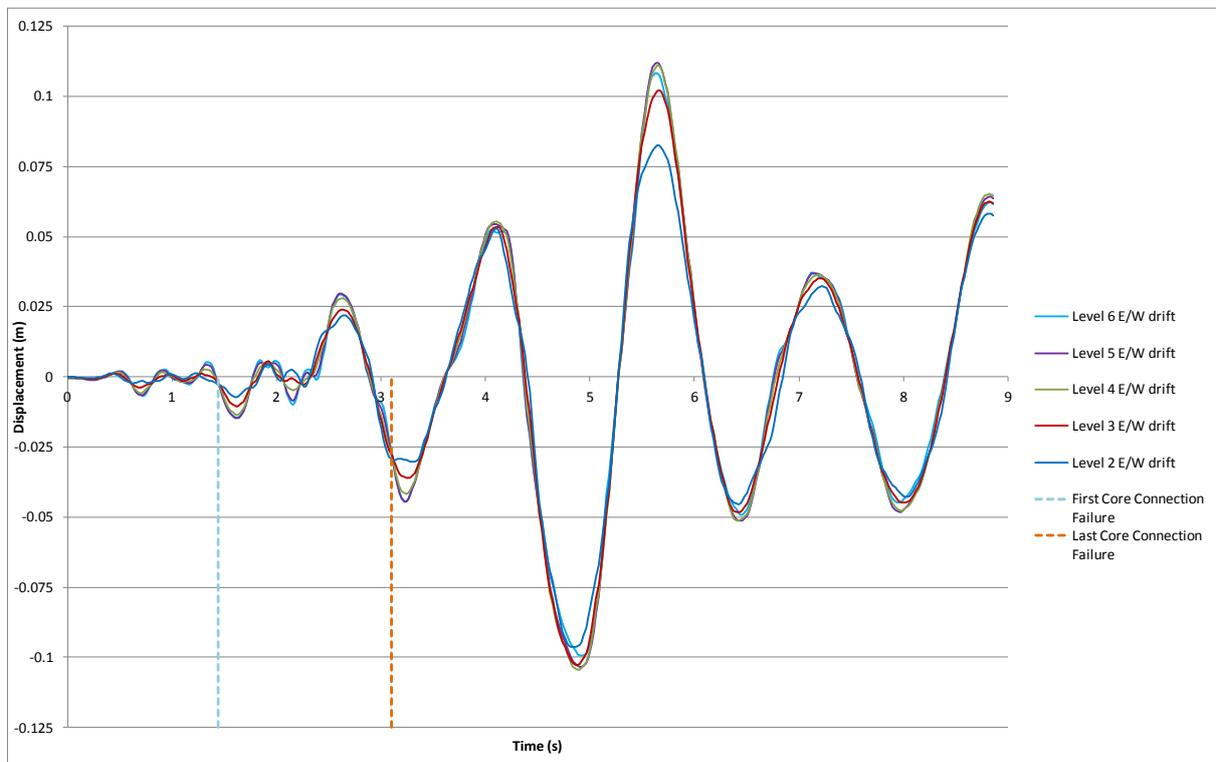
**Figure G.5: Frame 1 east/west inter-storey displacements.**
