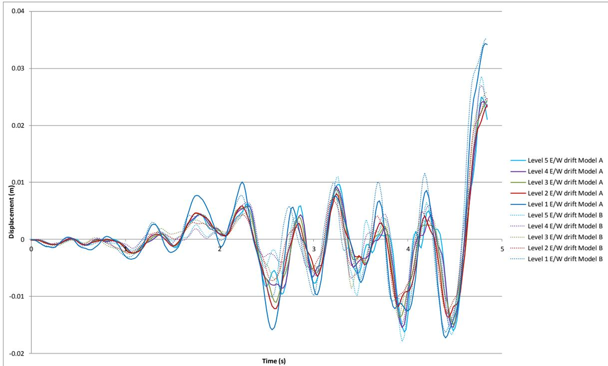
**Figure I.6: Frame 4 east/west inter-storey displacements.**
