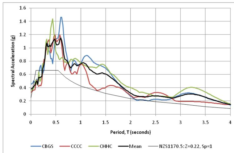
**Figure 25: Lyttelton N90E 5% damped response spectra (east/west)**
