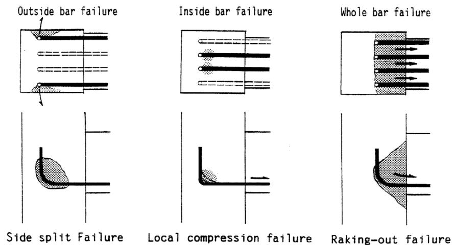
**Figure B.3: Hooked anchorage failure modes (from [21])**
