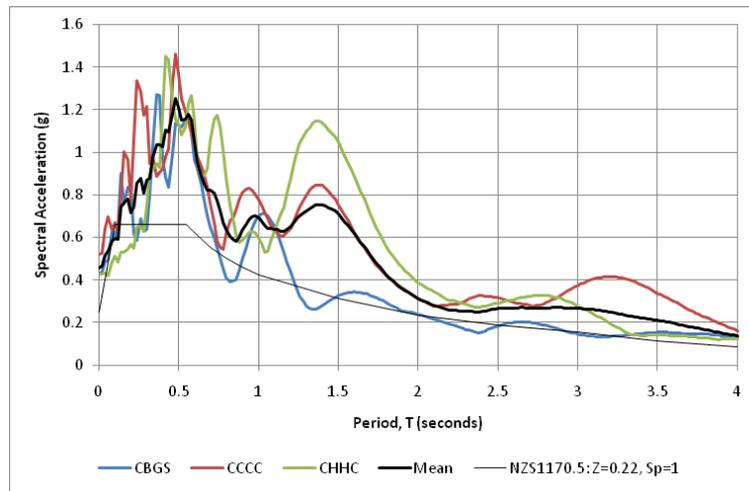
**Figure 24: Lyttelton N00E 5% damped response spectra (north/south)**
