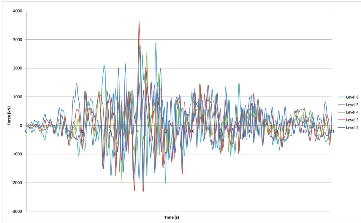
**Figure F.14: North core Slab 4/C to C/D diaphragm north/south actions.**
