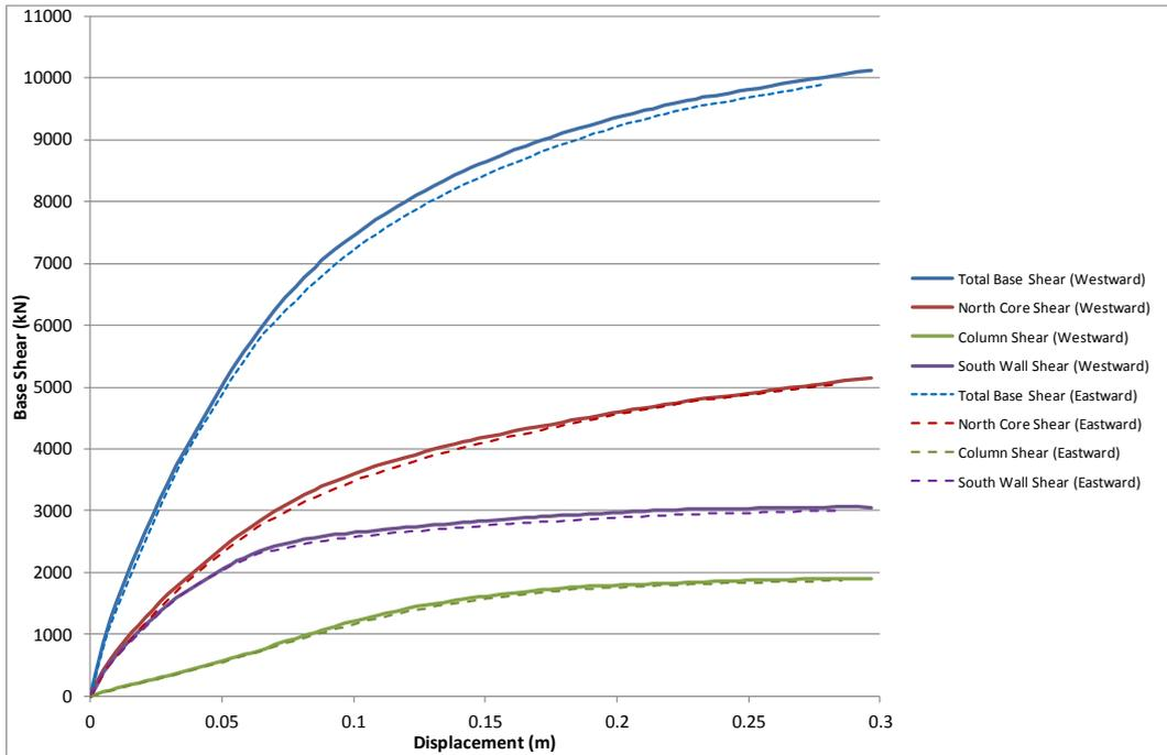
**Figure 29: Model A base shear components - east/west direction.**
