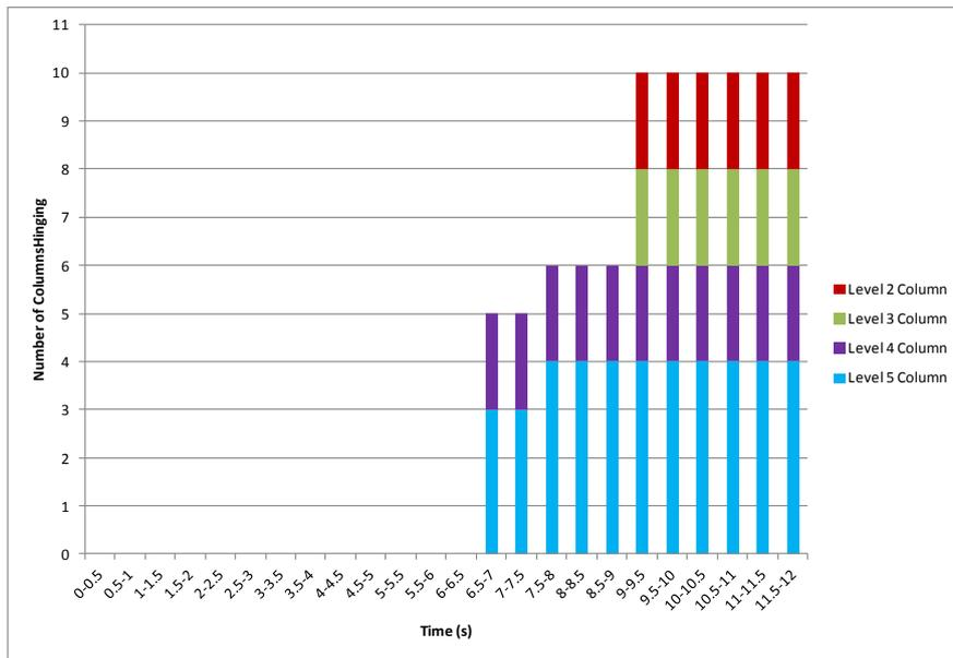
**Figure 43: Column hinge progression - Darfield, Model A.**
