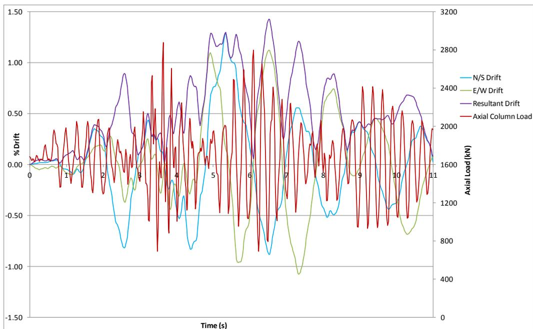
**Figure 56: Column D2 Level 1 axial load and drift plot - CBGS, Lyttelton**
