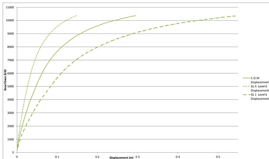
**Figure 31: Model A Level 6 western pushover displacement profile.**
