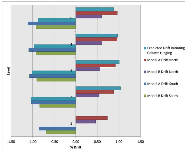
**Figure 39: Frame F north/south storey drifts - Darfield.**
