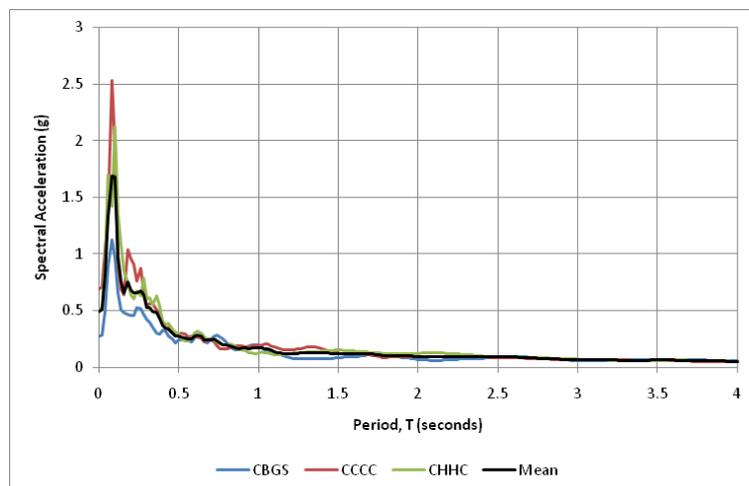
**Figure 26: Lyttelton Vertical 5% damped response spectra**
