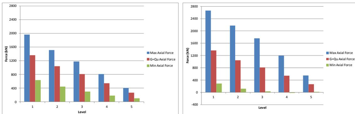
**Figure 55: Column 4 D/E axial load variation - CBGS (left) & CCCC (right), Lyttelton**
