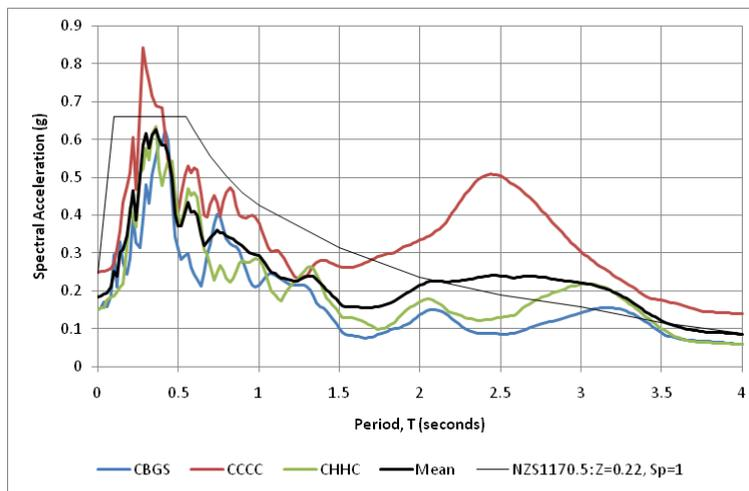
**Figure 22: Darfield N90E 5% damped response spectra (east/west)**
