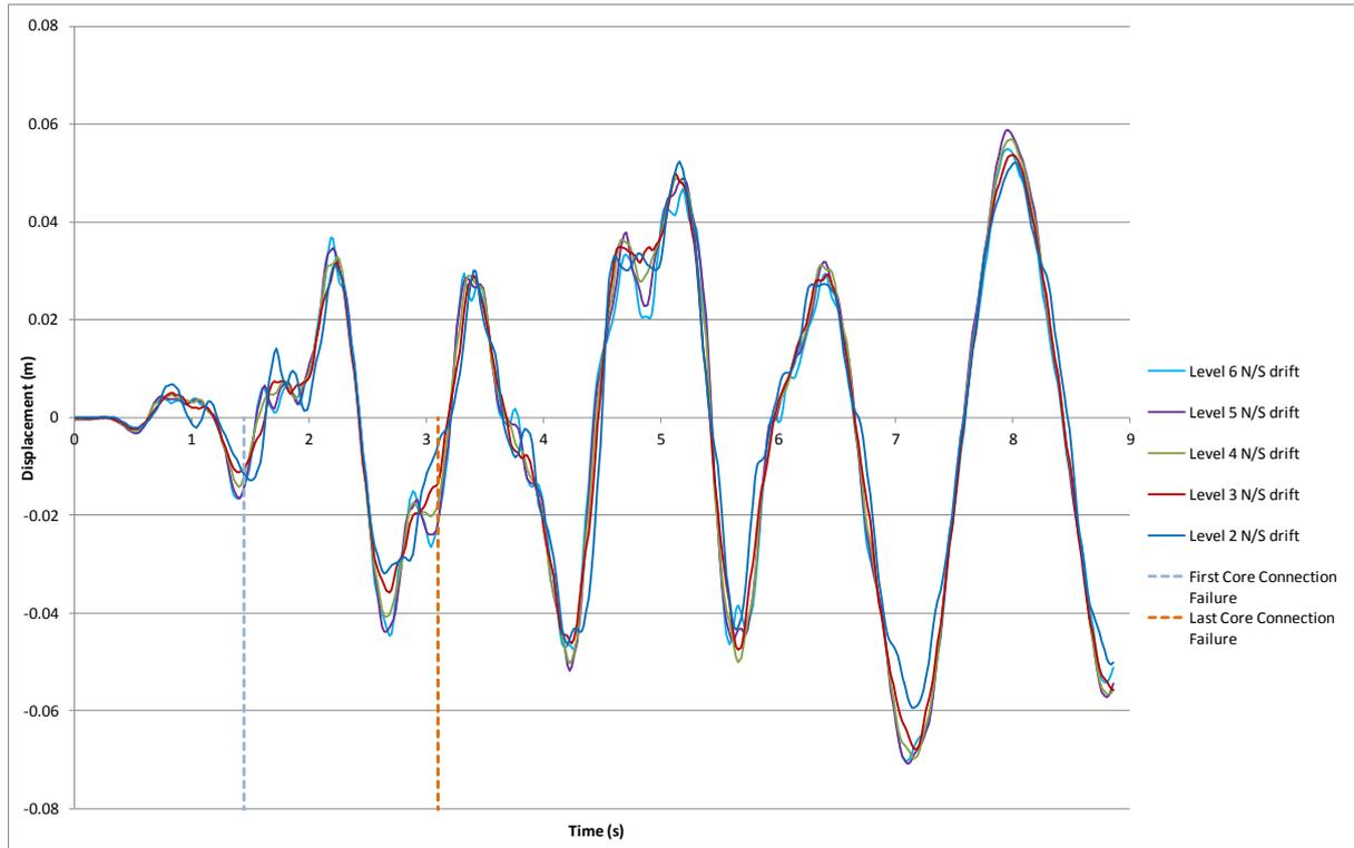
**Figure G.4: Frame F north/south inter-storey displacements.**
