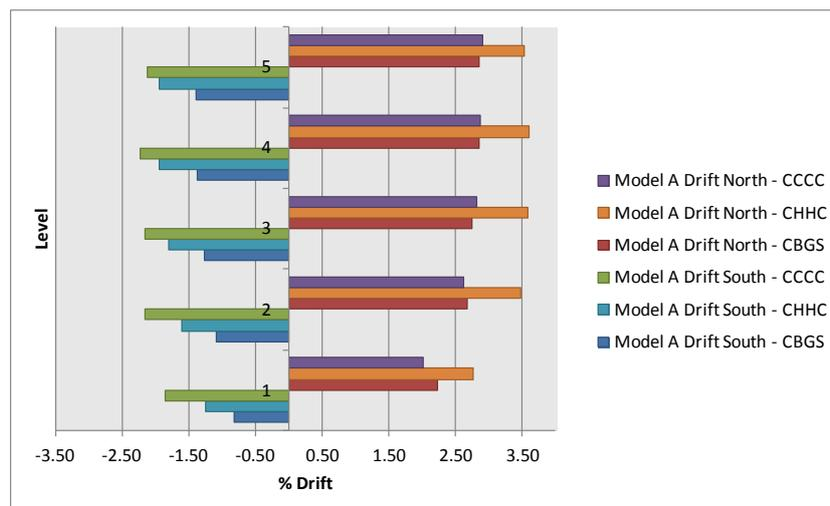
**Figure 45: Frame A north/south storey drifts - Lyttelton.**
