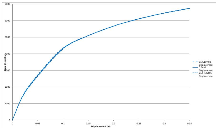
**Figure 33: Model A Level 6 northern pushover displacement profile.**
