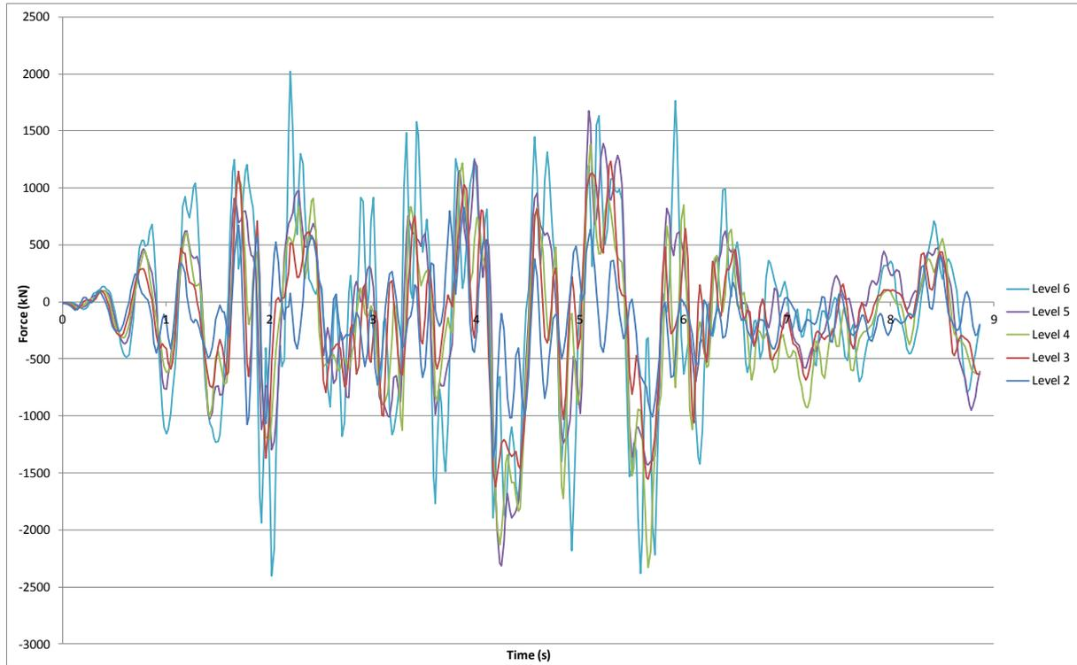
**Figure G.17: North core Wall 5 diaphragm east/west actions.**
