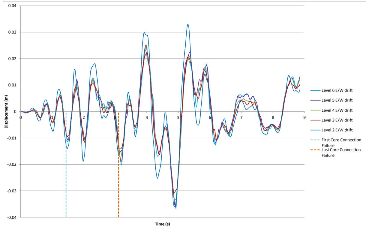
**Figure G.6: Frame 4 east/west inter-storey displacements.**
