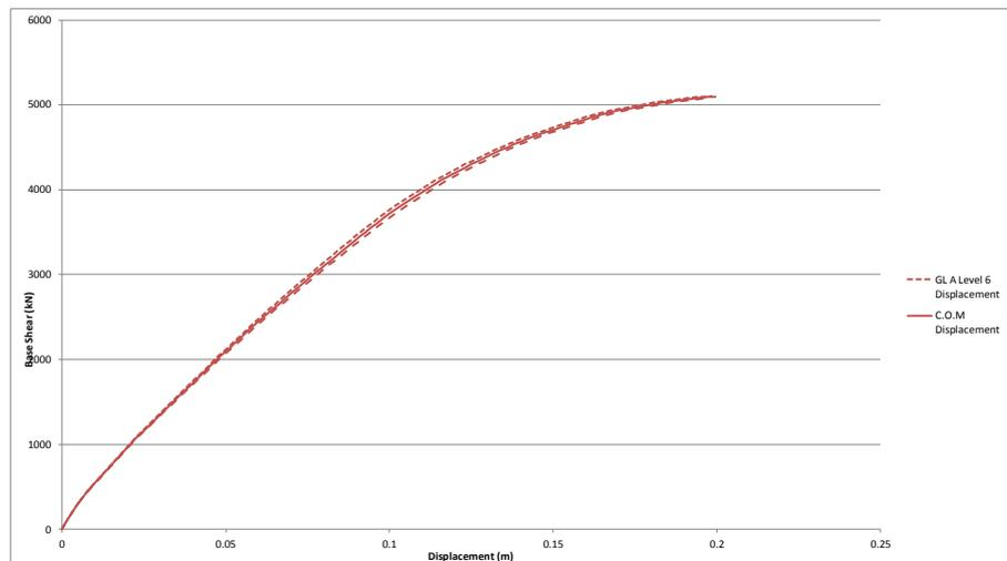
**Figure 34: Model A Level 6 southern pushover displacement profile.**
