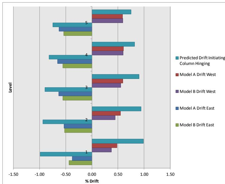
**Figure 40: Frame 1 east/west storey drifts - Darfield.**
