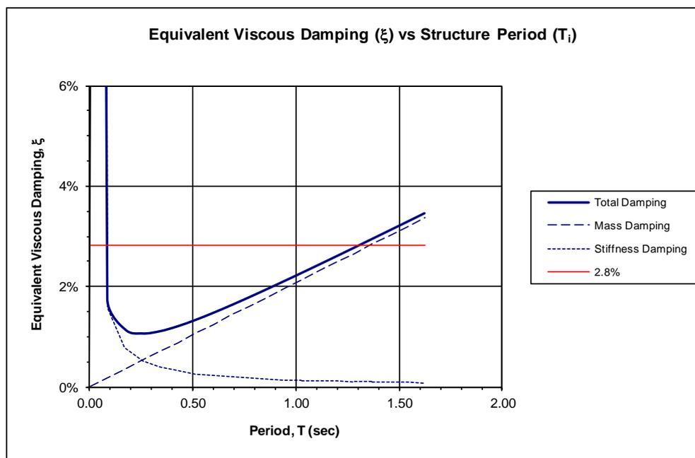
**Figure 27: Equivalent viscous damping vs structure period - Lyttelton**
