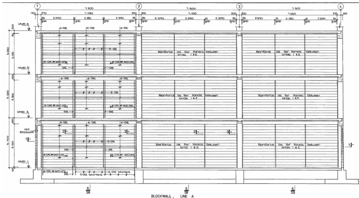
**Figure 15: Record structural elevation of masonry infill panels [1]**
