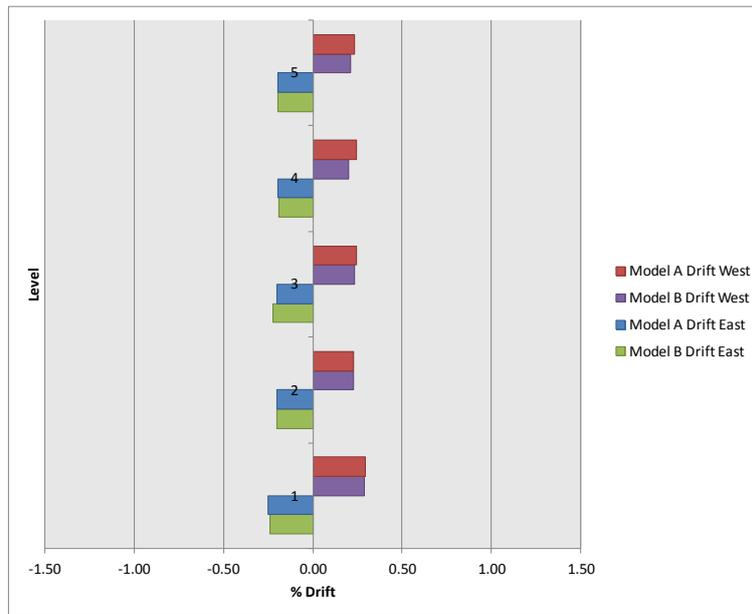
**Figure 41: Frame 4 east/west storey drifts - Darfield.**
