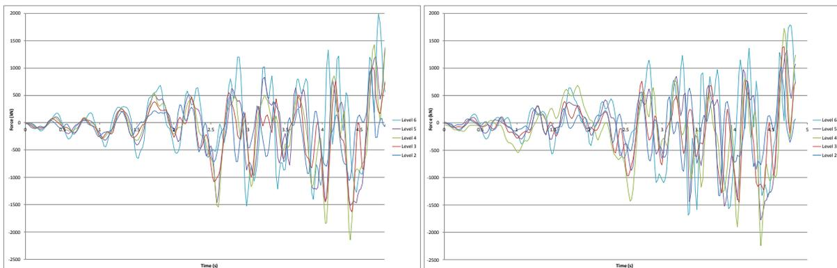
**Figure I.18: North core Wall 5 diaphragm east/west actions (no masonry left, with masonry right).**
