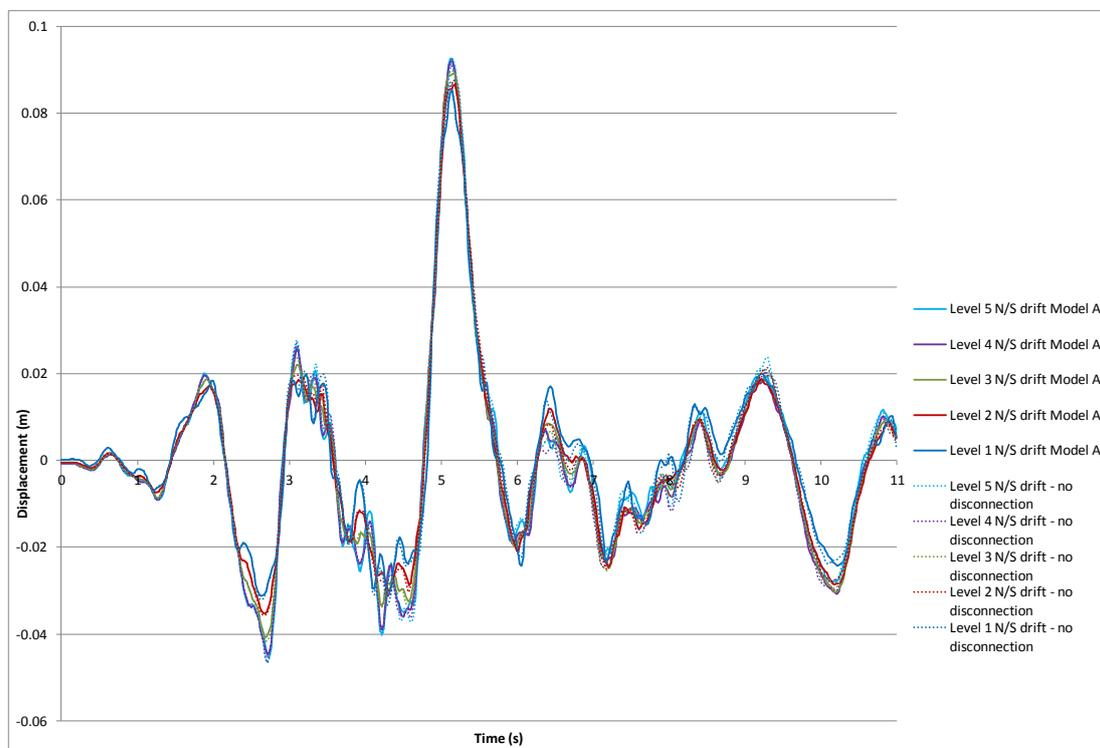
**Figure J.3: Frame A north/south inter-storey displacements.**
