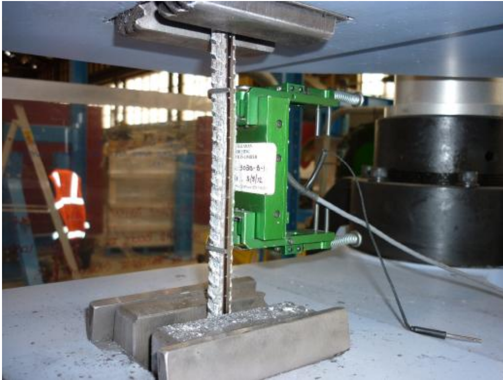
Figure 21 Tensile testing of steel sample
