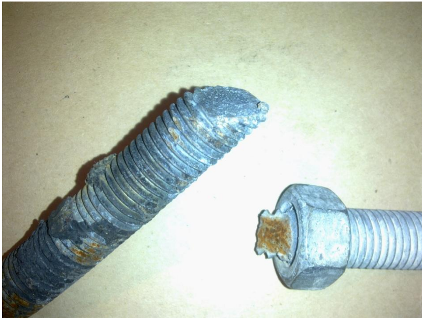
Figure 37 - M20 Drag Bar Bolts (Portions shown are from two different bolts) (left to right) (a) Grey portion with smooth diagonal end had epoxy residue from slab indicating it was cut this way prior to installation; (b) Necked and dimpled fracture surface at underside of bolt typical of direct tensile fracture in threaded rods.
