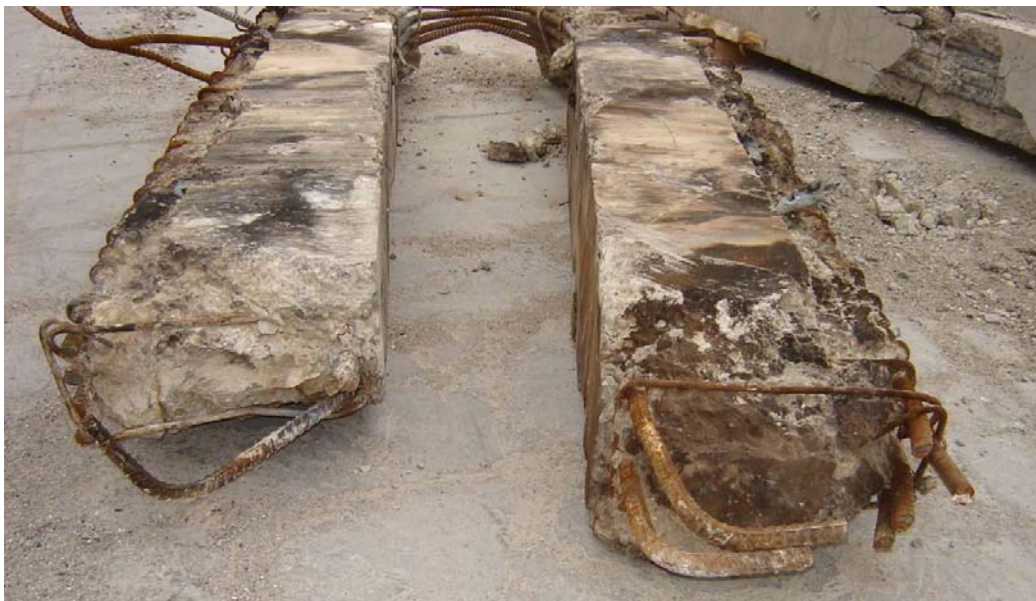
Figure 12 - Interior Pre-cast Log Beams from Line 2 and 3 (DENG Section 3 Dwg S15 (Figure 66)) showing smooth concrete formed for beam-column joint and bottom hooked bars that have pulled out of beam-column joints without any obvious straightening; metal decking has pulled away from slab seating; no slab remains attached to the beams
