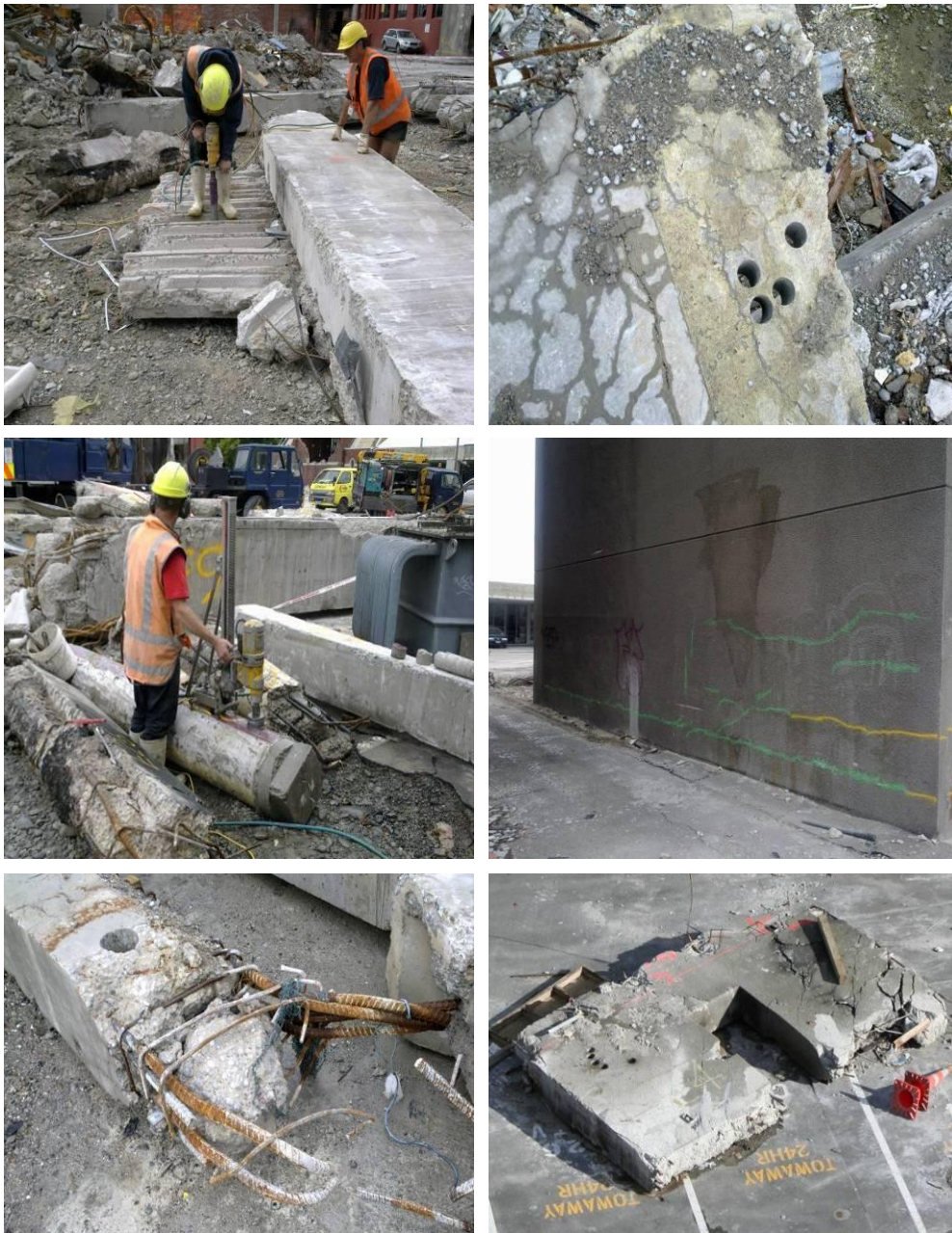
Figure 46 – Locations of concrete cores taken for testing (clock-wise from top left) (a) Slab attached to Line 1 or 4 perimeter shell beam (Item E23) (b) Slab attached to Line 4 perimeter shell beam (Item E14); (c) Line 5 shear wall through stair well at Level 1; (d) Line 1 South wall Level 4 to 5 (Item E4); (e) Pre-cast log beam from Line 2 or 3; (f) Level 6 400 mm diameter column (Item E25)
