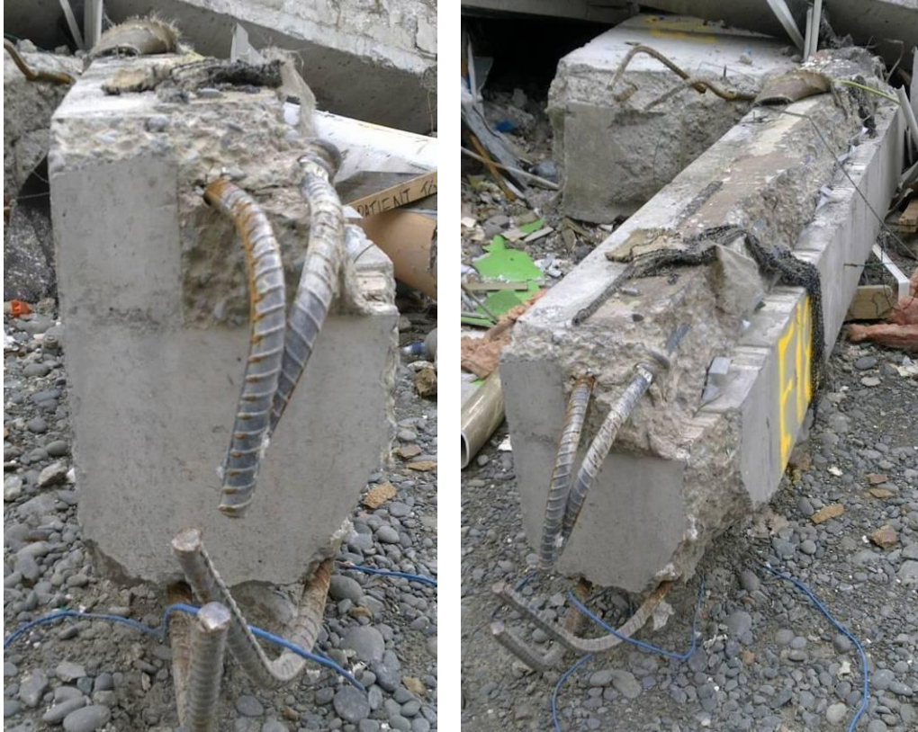
Figure 13 - Item E18 Pre-cast edge beam north-west corner (DENG B22 Dwg S18 (Figure 67) (from left to right) (a) Smooth form finish at attachment to column 4A (DENG Detail I Dwg S19 (Figure 70)); (b) No starter bar reinforcing steel extended from this pre-cast beam into slab. This was consistent with what was shown on the Drawings (DENG Section 4 Dwg S15 (Figure 66).
