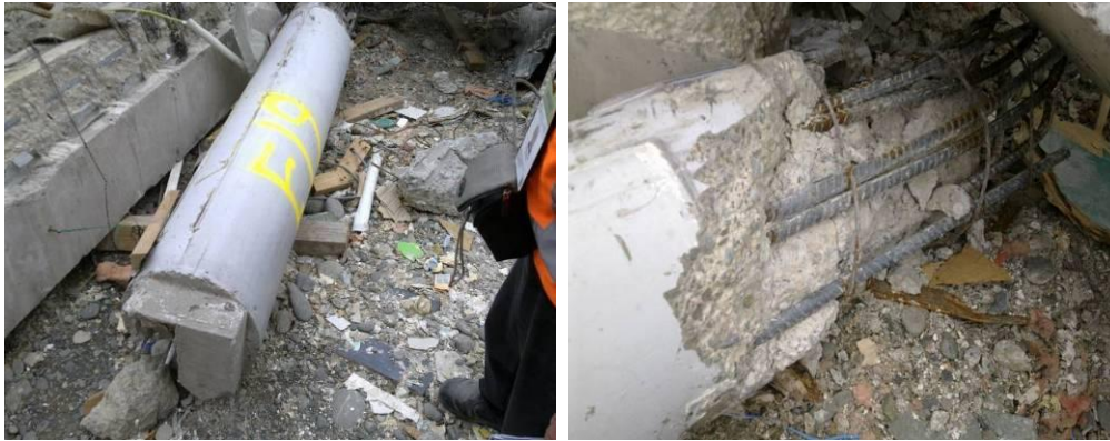
Figure 9 - 400 mm diameter column Item E19. (Left to right) a) Level 6 to Roof, likely location Grid F (Figure 65) based on roof steelwork hold down attachment detail; b) Flexural fracture at base in lap zone of vertical reinforcing steel. R6 spirals at 250 centres can be seen (Figure 69).
