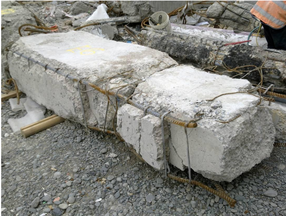
Figure 6 - Edge shell beam Item E6 showing unreinforced concrete infill and smooth interface between shell beam and in-fill. The DENG Specification Precast Concrete cl 3.12 required roughened interface surfaces (Figure 77).
