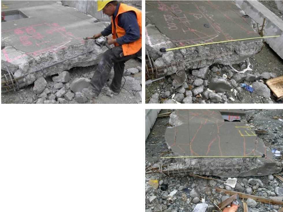
Figure 43 - H28 from east and west end of Line 1 South Wall Item E1 (clockwise from top left) (a) H28 about to be cut from east end (E1E); (b) Top of 1000 mm long E1E sample 1300 mm from top of L2 slab; (c) Top of 1000 mm long E1W sample from west end 750 mm from top of L2 slab. Coupling beam depth was 1700 mm.
