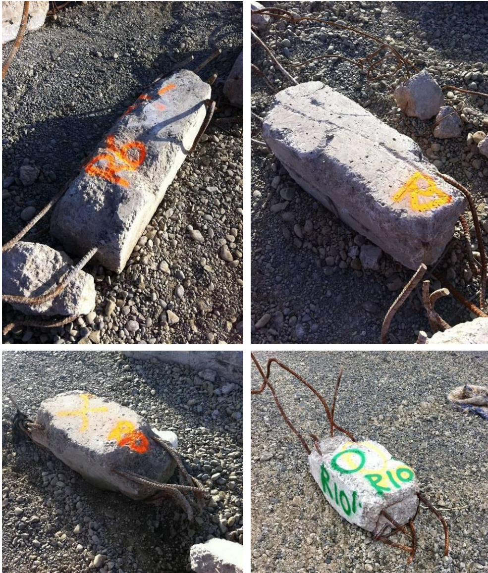
Figure 56 -400 x 300 mm Rectangular Columns (from left to right and top down) (a) tR6 base at far end connected by reinforcing to (b) tR7 below, with beam-column joint failure; (c) tR10 remnant; (d) tR10' remnant
