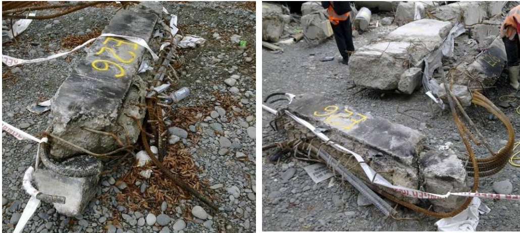
Figure 11 - Interior Pre-cast Log Beam from Line 2 and 3 (DENG Section 3 Dwg S15 (Figure 66)) (left to right) (a) Diagonal shear damage at end and smooth formed surface at beam-column joint; (b) Mid-portion of beam concrete has broken away and stirrups are pulled apart.
