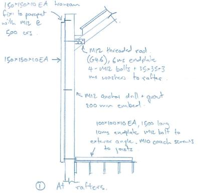
lookiookio EA, Miz bolt to exterior angle and 5-Miz anchors drilled and grouted into brick.
