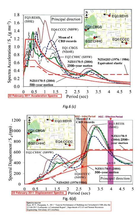
Figures 6(a), (b), (c) and (d) show acceleration and displacement spectra as recorded at 4 locations around the central business district for the 4 September event and the 22 February events. Only the principal direction of motion at each location is shown (the ground motion is normally recorded in two orthogonal directions, and one vertical). For analysis of the Hotel Grand Chancellor average values have been used to determine the response of the structure.
