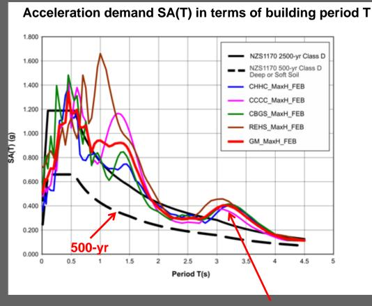
**500yr = Design-level for** normal-use structures Z=0.22 **2500yr = Design-level for** post-disaster essential facilities RZ=1.8\*0.22=0.40 Red curve = geometric mean for the four sites
