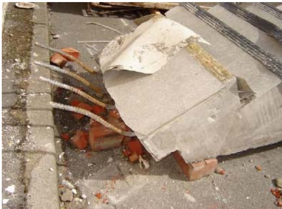
Figure 7.3 : Top Starters Pulled Out
