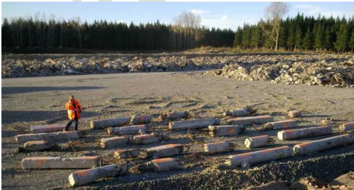
Figure 42 CTV Columns remnants extracted from the Burwood Landfill CTV debris (at right) for Schmidt Hammer testing and coring. Full height and partial height remnants can be seen.
