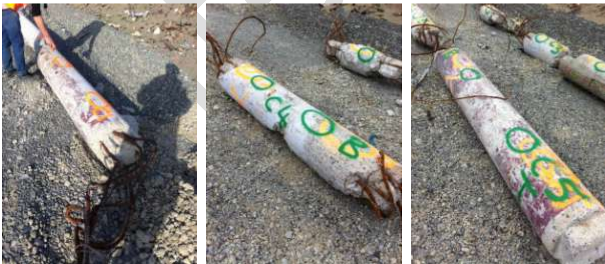
Figure 43 400 mm diameter columns full height (left to right) a) Test Item C1 Level 6 to roof column with base hinging failure, still connected by reinforcing to C8 below; b) C4 hinging top and bottom; c) C5 Level 6 to roof column with hinging at base.
