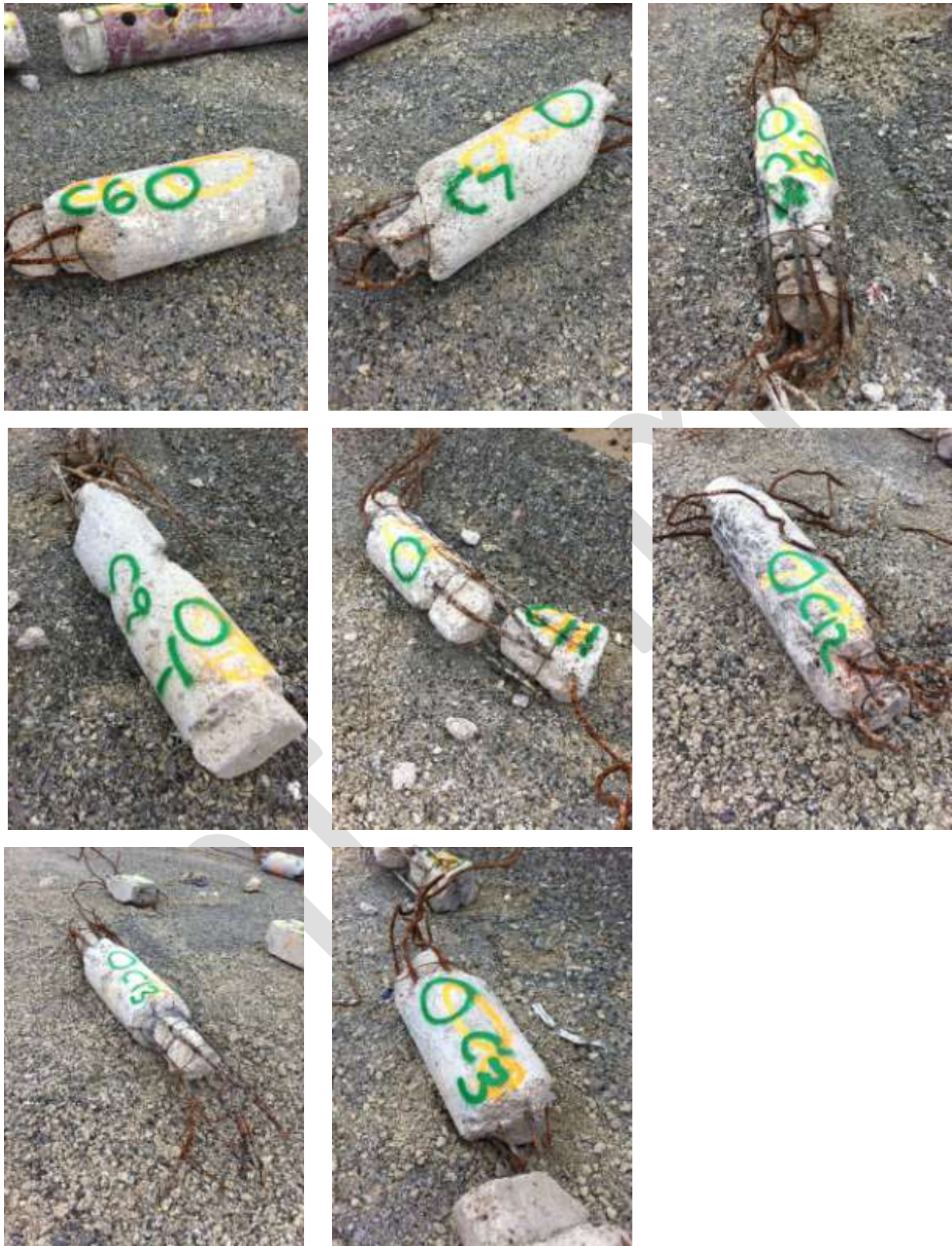
Figure 46 400 mm Diameter Columns at Burwood showing similar base and/or mid-height failures (Left to right, top row down) a) Test item C6 Level 6 column head with mid-height failure; b) C7 with base and mid-height failures; c) C8 with base flexural (near end) and mid-height spearhead failures; d) C9 Level 6 column head with mid-height failure; e) C11 base (near end) and mid-height failure; f) C12 base and mid-height failure; g) C13 base and mid-height flexural failure (near end); h) C3 similar to C13 but lower bars have been cut during de-construction at start of spalling.
